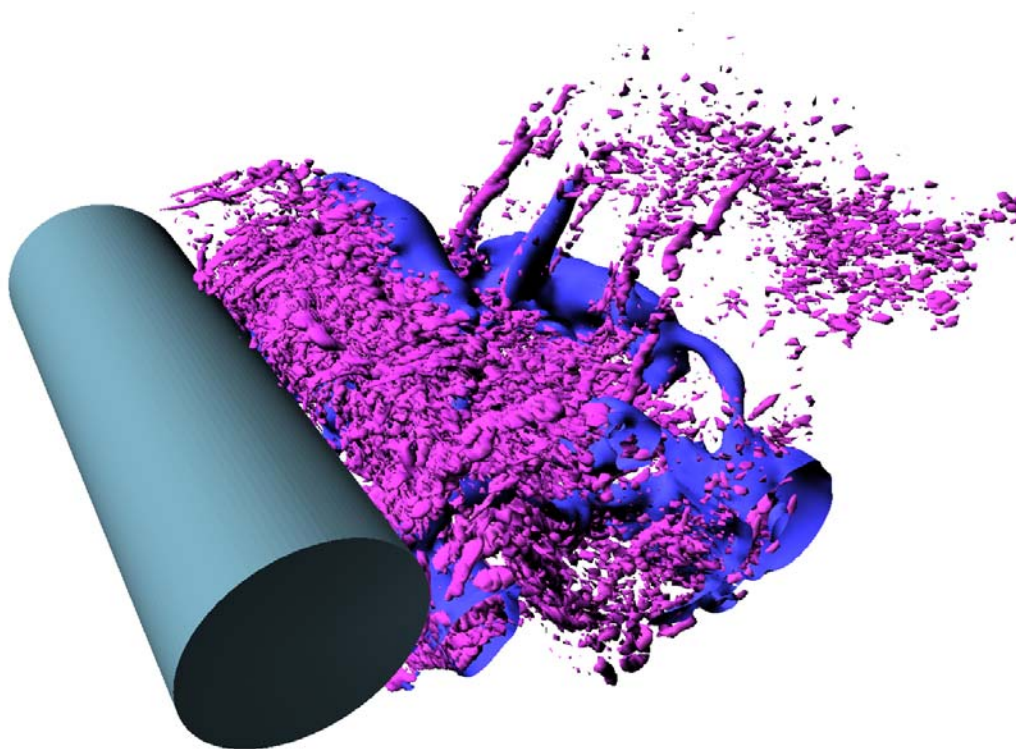
Fig. 4.3: Isosurfaces of a specific pressure fluctuation P'/\frac{1}{2}\rho U_\infty^2 = -0.5 , darker gray, and of Q = 25.0 , lighter gray. (LES1 smago).
