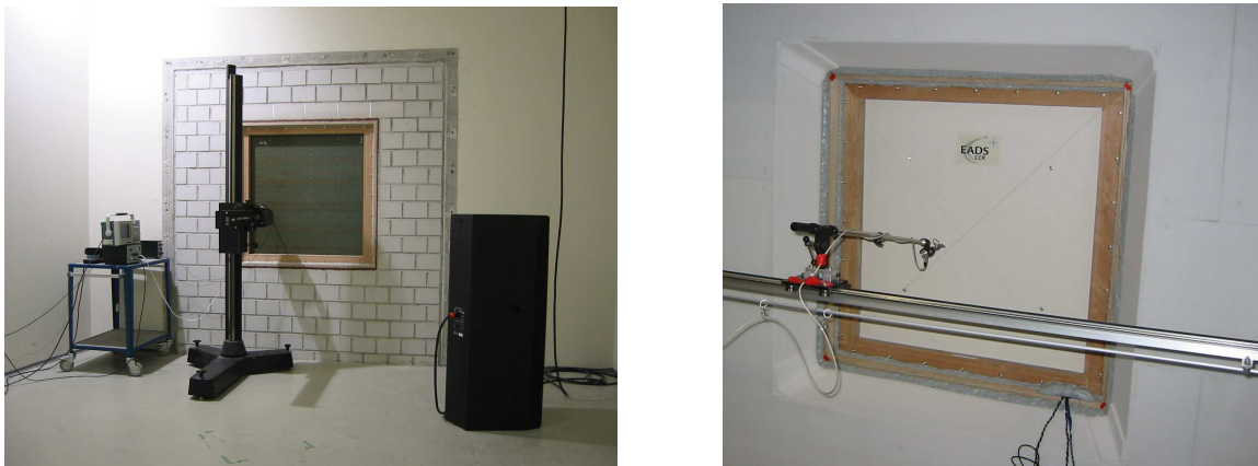
Figure 5.10: Transmission loss test window (view from the reverberation room on the left side and view from the anechoic chamber on the right side)
