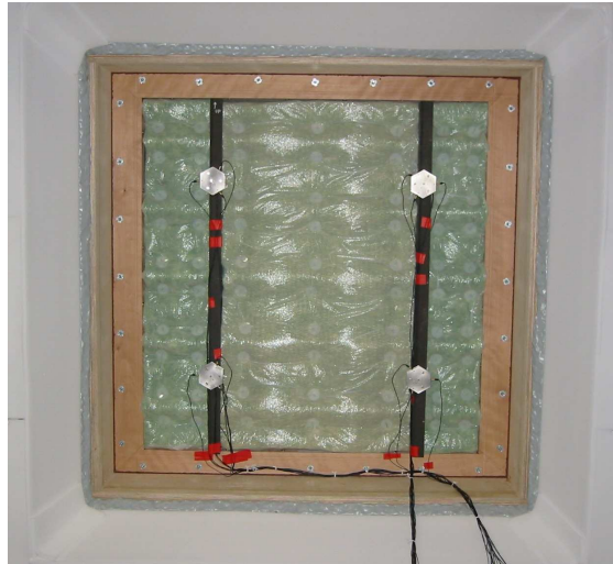
Figure 5.8: Fuselage panel installed in TL test suite, active attachment elements already installed
