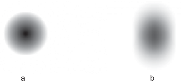
Figure 6: Illustration of the picture of a bead recorded by a CCD-camera: a) In the case of a resting particle results a point-symmetric distribution of brightness. b) In the case of a vertically oscillating particle, the distribution of brightness is smeared out in this direction.
