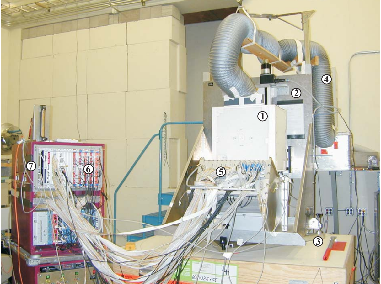
Figure 6.8: Setup of MEGA at Duke: The MEGA prototype (1) is located below a Styrofoam housing to regulate the temperature via an air-conditioning system (4). MEGA is mounted on an XY-table (2) to scan the detector with the narrow pencil beam. To verify the field of view, the whole XY-table assembly can be rotated (3) around the center of the tracker. The data acquisition system (front-end (5), ADCs (6), CPU (7)) is also shown.
