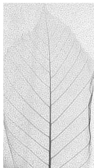
Fig. 3.84: Reconstruction of the projection shown in Fig. 3.83 by help of a Wiener filter. The blur due to the geometry of the neutron beam and detector blur is removed. The SNR is 20.6.
