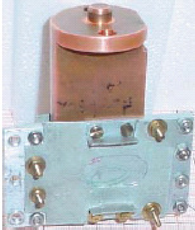
Figure 4.4: Picture showing the EuS sample and the sample holder used for SAPNS experiments.
