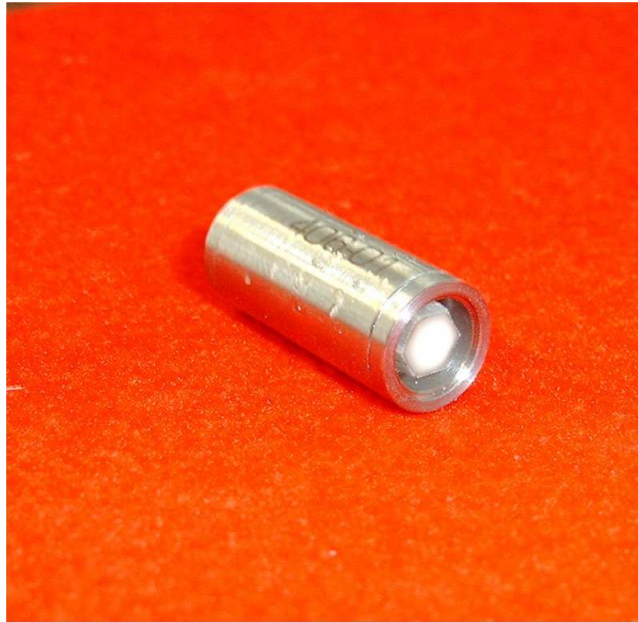
Figure 5.8: Photo of the lens in steel enclosure
