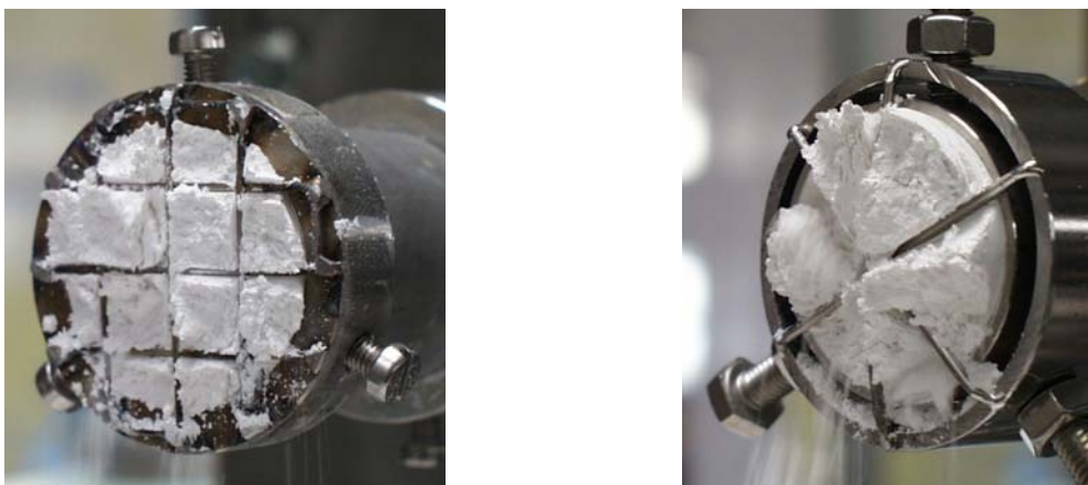
Fig. 4-27: Powder coming out of the grid attachment (left) and the star attachment (right)
