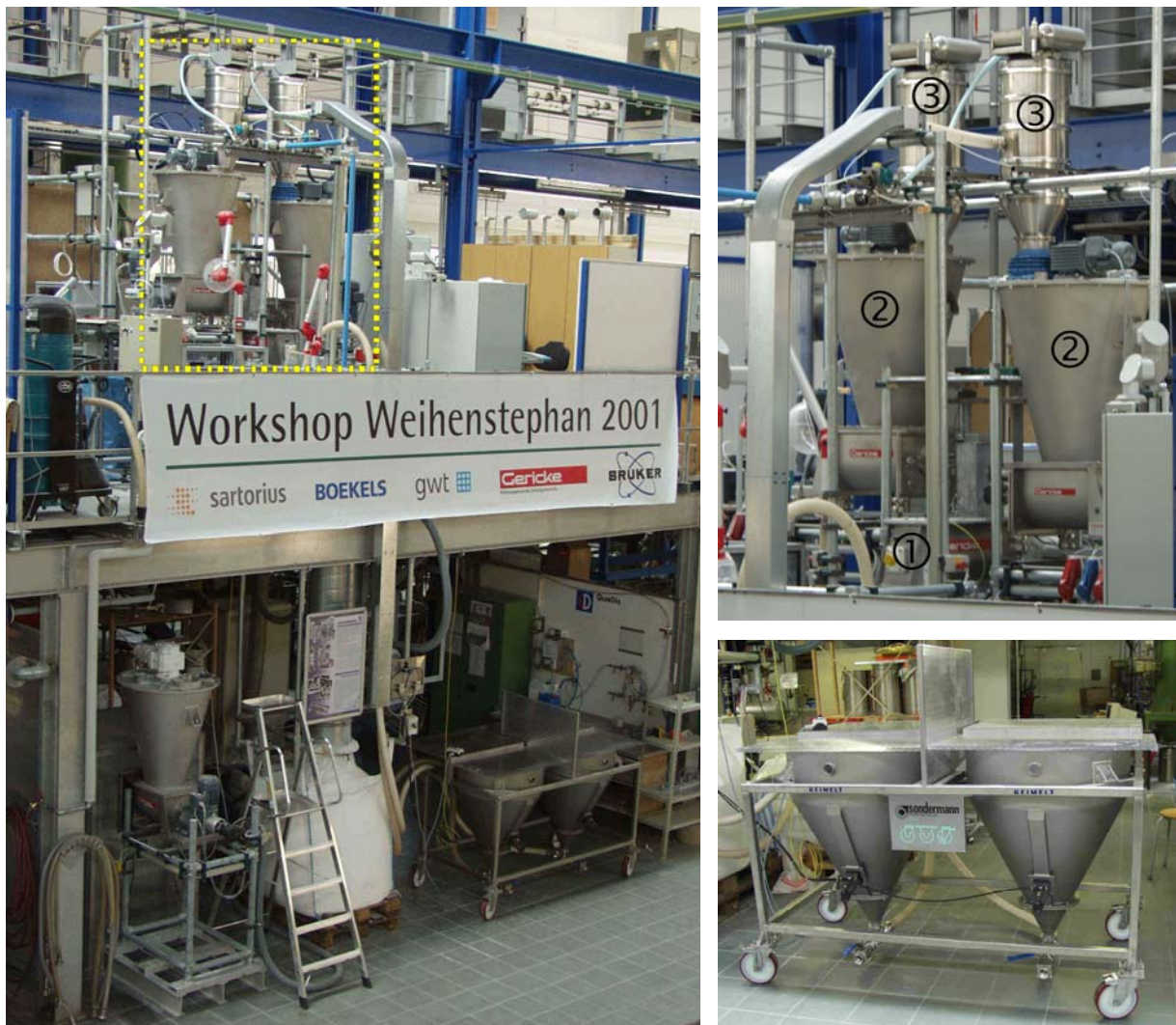
Fig. 4-1: Front view of the experimental rig: ① continuous mixer, ② volumetric feeders, ③ suction conveyors
