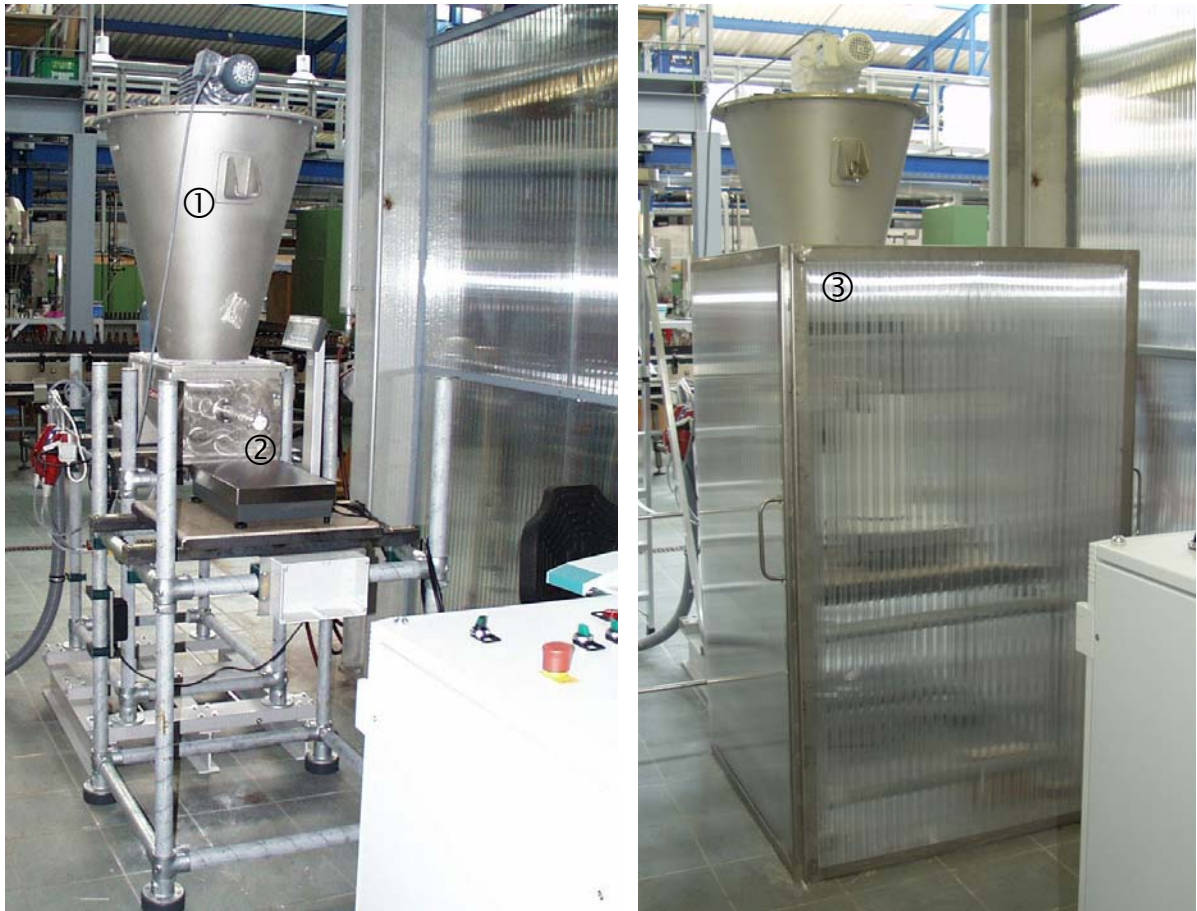
Fig. 4-24: Trial equipment used for the dosing experiments: Volumetric feeder ①, balance ② and plastic housing ③
