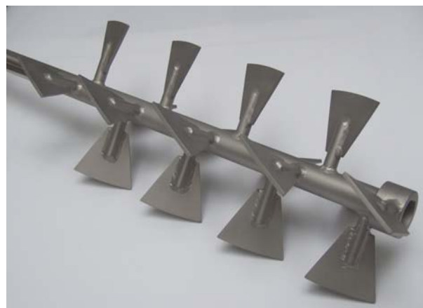
Fig. 5-9: Mixing device to be tested in the future: Increased number of paddles fixed on a shaft
