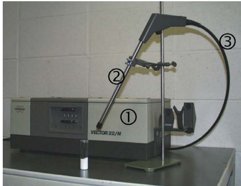
Fig. 4-63: FT-NIR spectrometer VECTOR 22/N from the company Bruker Optik GmbH (① spectrometer, ② probe, ③ glass fiber cable)
