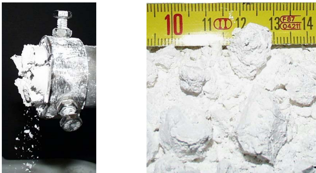
Fig. 4-34: Calcium carbonate powder compacted due to the use of a star attachment
