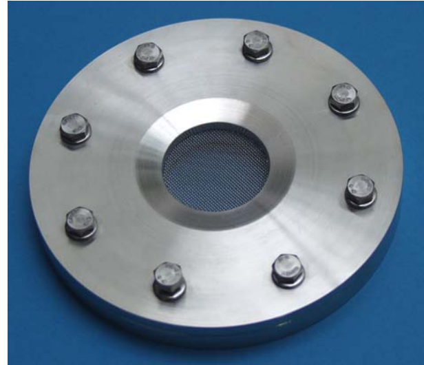
Fig. 4-93: Sieve attachment for the self-constructed calibration apparatus (to be put on the inlet for samples to be analyzed, compare © in Fig. 4-89)
