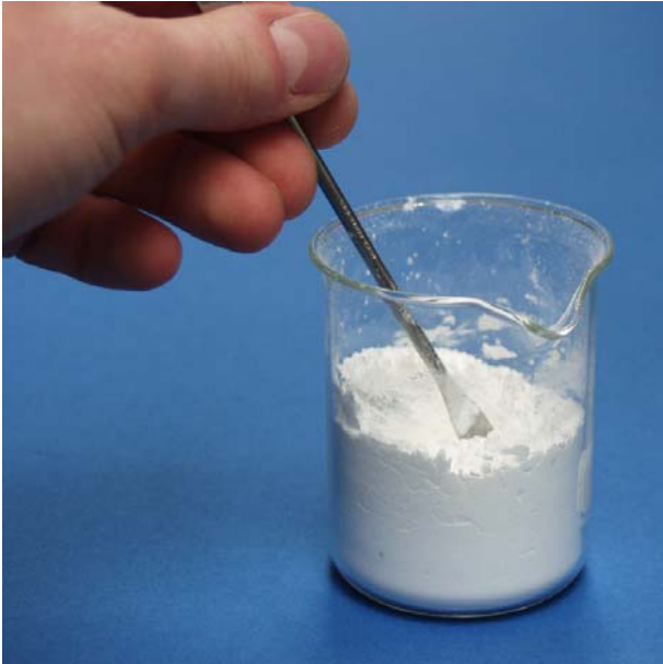
Fig. 4-94: Sample preparation by mixing the powders in a beaker with a spatula
