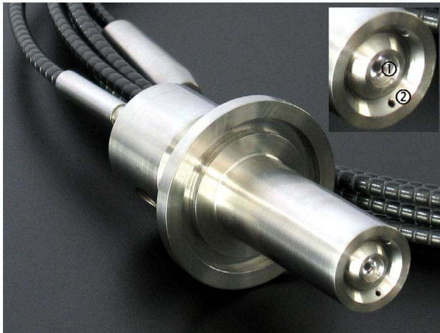
Fig. 4-86: NIR probe from the company Precision Sensing Devices, Inc. that uses compressed air for cleaning the probe tip (enlarged probe tip: ① window for NIR light, ② drilled holes for air-cleaning) [Courtesy of Bruker Optik GmbH]
