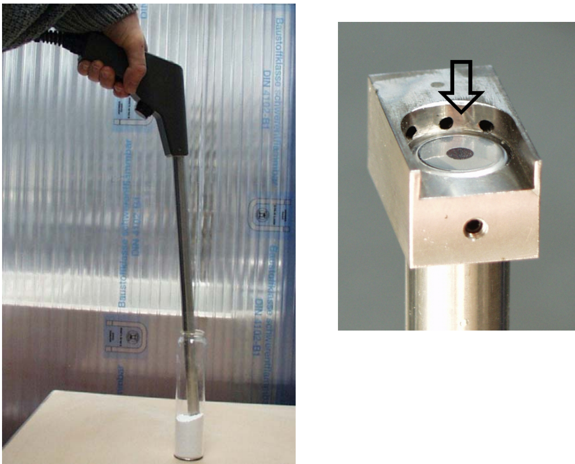
Fig. 4-87: Possibilities to calibrate the FT-NIR spectrometer VECTOR 22/N: Immersing the probe into the powder mixture (left), putting powder on the tip of the NIR probe by using the developed attachment (right)
