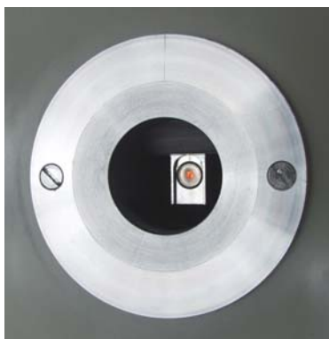
Fig. 4-90: Self-constructed calibration apparatus: View in the inlet for the samples to be examined (compare ③ in Fig. 4-89)
