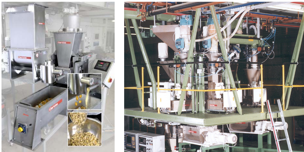
Fig. 1-1: Continuous mixer GCM 500 with a mixing chamber volume of 15 l from the company Gericke (left) and continuous mixing installation (right) [Courtesy of Gericke AG]
