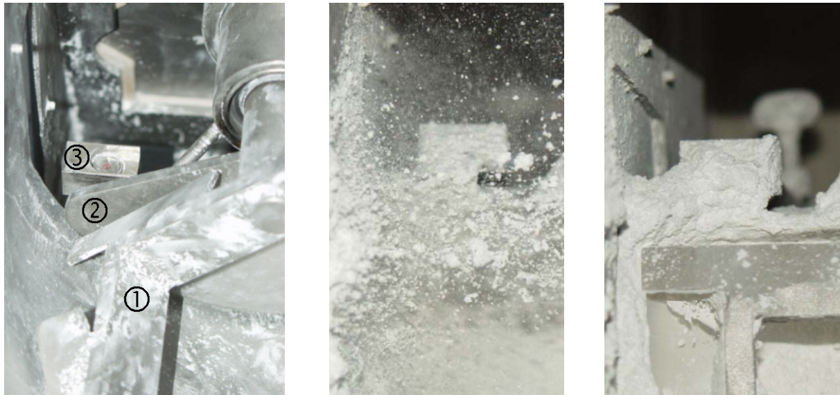
Fig. 4-85: In-line concentration determination in the outlet of the continuous mixer GCM 500 from the company Gericke (left: empty mixer with ① mixing device, ② half-closed weir and ③ NIR probe with developed attachment for air-cleaning; middle: filled mixer and rotating mixing device; right: filled mixer and stopped mixing device)
