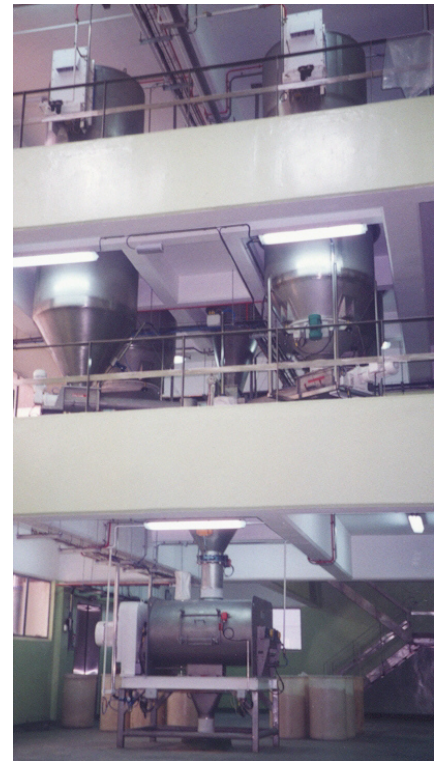
Fig. 1-2: Discontinuous mixer GMS 5 000 with a mixing chamber volume of 5 000 l from the company Gericke (left) and discontinuous mixing installation (right) [Courtesy of Gericke AG]
