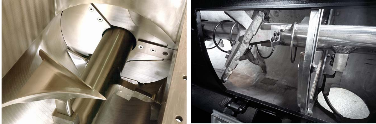
Fig. 5-12: Different mixing devices available for the continuous dynamic mixers from the company Lödige: Plowshares (left) and blades (right) [Courtesy of Gebrüder Lödige Maschinenbau GmbH]
