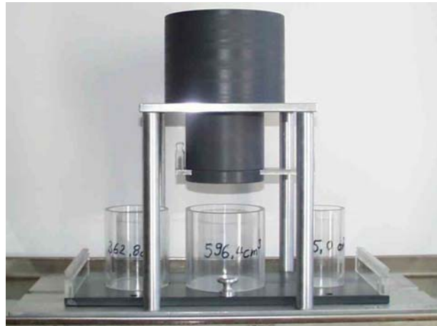
Fig. 4-8: Device to determine the bulk density
