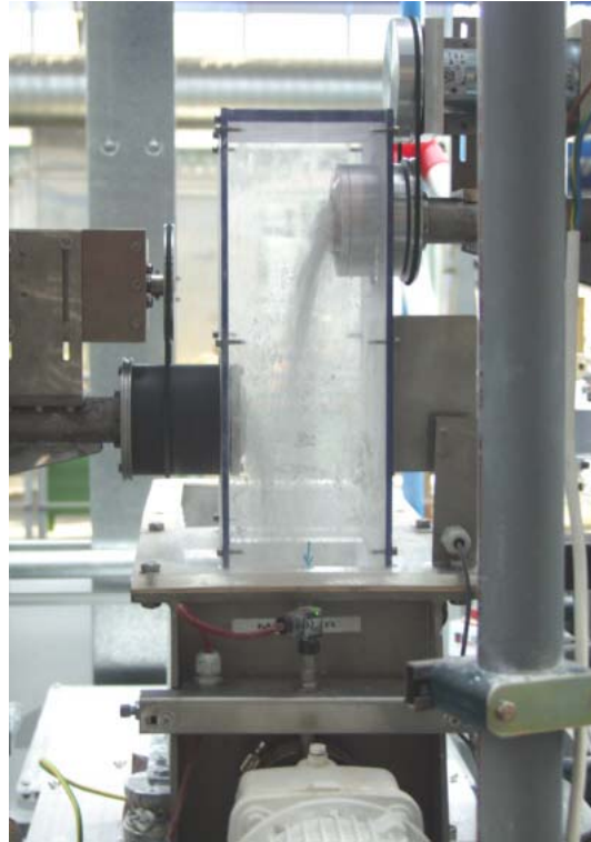
Fig. 4-53: Powder dosing in the continuous dynamic mixer: Maize starch (left) and calcium carbonate (right)
