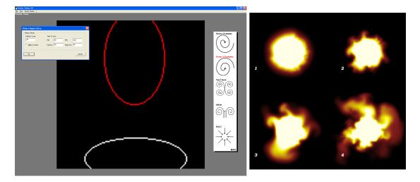
Figure 4.13: The left image shows the user interface to define regions for automatic insertion of templates. In the four right images, templates of equal shape and number are inserted. In images 1 to 3 we see high, medium, and low frequency structures. In image 4 all frequencies are contained. These effects are achieved by using different lifetimes and scale factors.
