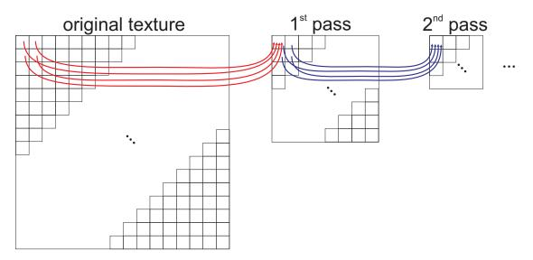
Figure 3.5: Schematic illustration of the reduce operation.
