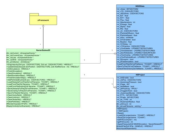
Figure 4.8: This figure shows a simplified UML diagram of the 2D Navier-Stokes classes. Note the connection to the clFramework (see Figure 3.10 for details) and the data storage classes colored blue.
