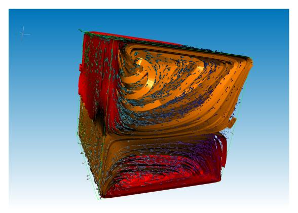
Figure 7.13: A 3D flow simulation with different forces driving on the top and on the bottom of the domain. The flow is visualized with a combination of stream ribbons and oriented particle splats.
