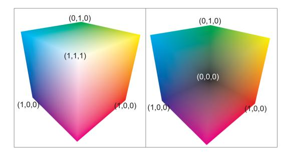
Figure 5.10: Rendering front faces (left) and back faces (right) of the volume bounding box in order to generate ray directions and texture coordinates of the first intersection points.
