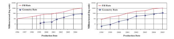
Figure 2.2: Pixel and Vertex performance of NVIDIA (left) and ATI GPUs (right).
