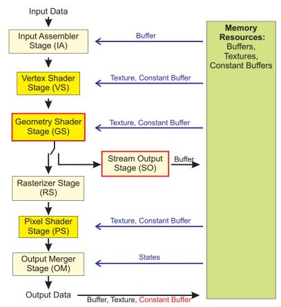
Figure 2.5: The Direct3D 10 Pipeline. Yellow boxes denote the three programmable stages. Important additions to the pipeline are marked in red.
