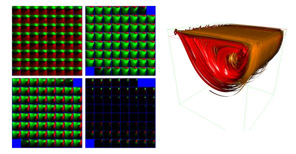
Figure 4.14: A flow inside a container with the lid moving at constant velocity. On the left the four atlases for pressure, x-, y-, and z-flow are shown. Positive values are color-coded in red, negative values are coded green. The right image shows a stream-ribbon visualization of the same simulation.
