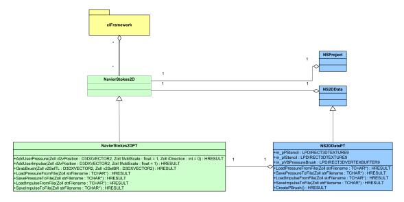
Figure 4.11: This figure shows a simplified UML diagram of the 2D Navier-Stokes classes supporting the flow templates.
