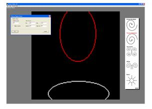
Figure 7.5: The WYSIWYG user interface to define regions for automatic insertion of templates. On the right, the iconic representations of the templates can be seen.
