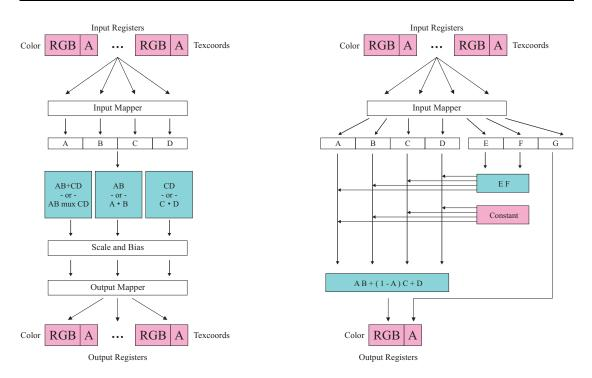
Figure 2.3: NVIDIA Register Combiners (simplified). The left image shows a general combiner while the right is a final combiner with restricted functionality. Depending on the GPU generation up to eight general combiners could be configured to work in a pipeline.
