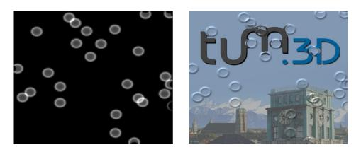
Figure 7.14: The 2D water demo. In the left image the result vector was rendered directly; thus, positive height values appear brighter. In the right image these height values were used to compute the refraction vector and this vector was used for a second texture fetch into a static environment map
