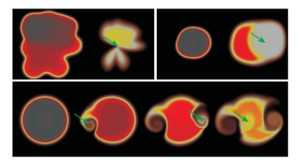
Figure 4.12: Effects of interactive template insertion are shown. The upper left image shows the effect of a sink template, in the right image a source template was applied. In the lower row an impulse template producing a vortex was inserted at different positions and orientations.
