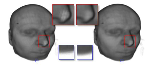
Figure 5.12: An MR data set visualized with SBVR (left) and the raycaster (right). Although the same step size was used, one can clearly see the superior image quality of the raycasted image. The red and blue squares magnify areas where the slice artifacts are particularly disturbing.
