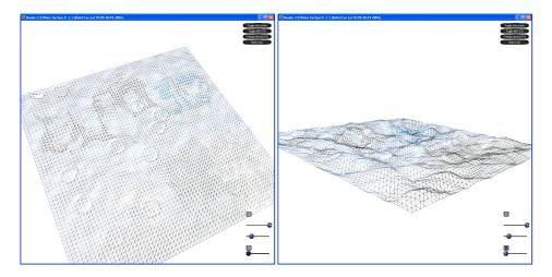
Figure 7.15: The 3D Water Demo. This program extends the functionality of the previous demo in such a way that a static triangle grid is displaced by the simulated height values.
