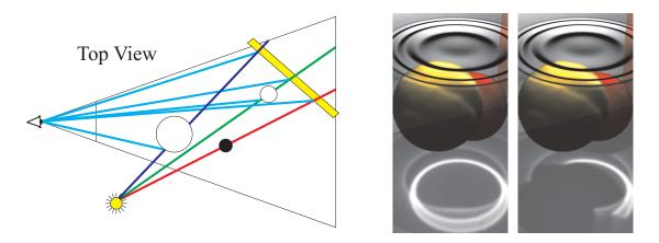
Figure 6.3: If a pixel shader illuminates all line-object intersections in view-space incorrect results are produced. In the example, five hits instead of three would be illuminated due to the black sphere being occluded in view space. In the two right images a scene is rendered without (left) and with (right) caustics shadowing. The artifacts can be clearly observed.
