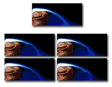
Figure 4.7: The images show a step flow. On top the static solution without vorticity confinement can be seen. In the four bottom images of the dynamic simulation with vorticity confinement is shown.
