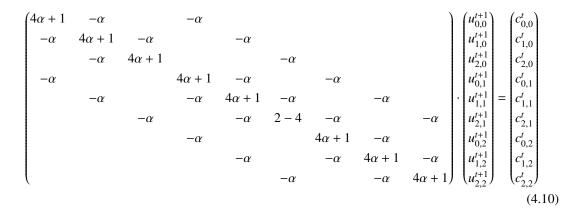
To solve this system of linear equations it takes more than a simple filter kernel. Using the linear algebra framework with the CG solver built-in ,however, only a few lines of code need to be changed. First the matrix has to be initialized differently. Therefore, it is sufficient to change the second line in Listing 4.1 to "float alpha = -(dT\*dT\*C\*C)/(h\*h), mainDiag=-4\*alpha+1;." Finally we replace the per fame iteration by the following code:
