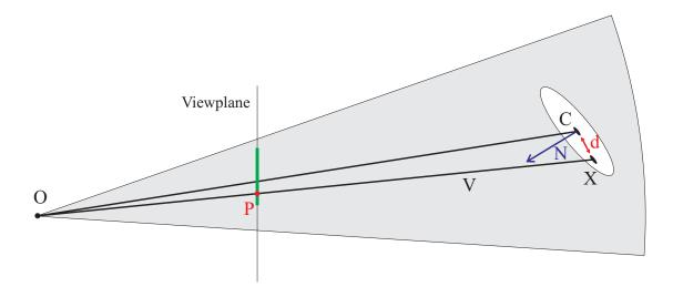
Figure 6.8: Schematic view of sprite-based raycasting. *P* is a pixel in the image plane, *O* denotes the viewing position and *d* is the distance of the intersection point to the receiver point. The distance is used to calculate the intensity. For a spherical intensity splat with size *s* and linear attenuation this is s - d.
