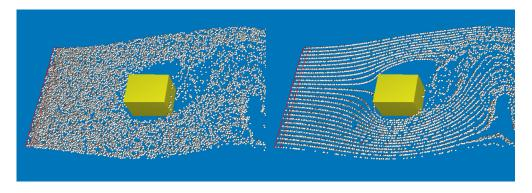
Figure 4.18: Random and Regular Distribution of Starting Positions Within the Particle Probe.
