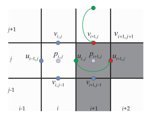
Figure 4.4: The image shows a staggered grid with the pressure values stored in the center of each cell, and the u and v components stored on the cell borders. This image also shows how the velocity values at obstacle (dark cells) borders are mirrored to match the border conditions.
