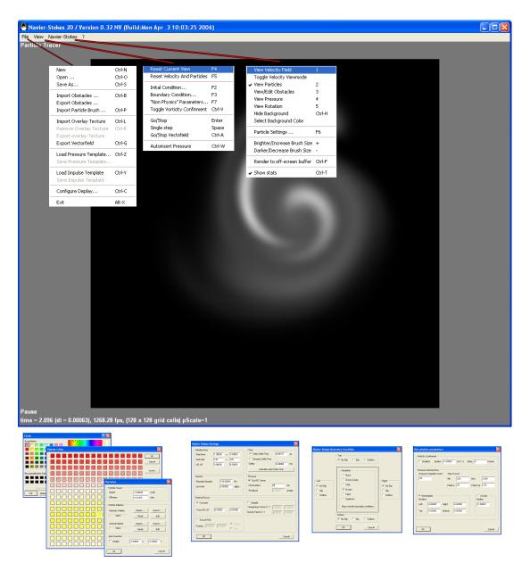
Figure 7.2: The basic UI of the "NavierStokes2D" application. The top image shows the screenshot of the program after startup together with the menu structure. The application allows the user to instantaneously interact with the flow, by inserting dye and adding external forces with the mouse.
