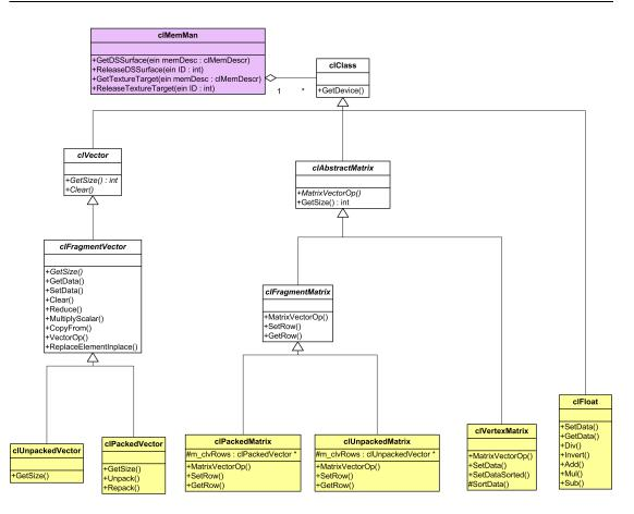
Figure 3.10: This figure shows a simplified UML diagram of the clFramework classes. The yellow classes represent the data types the user interferes with. Note the purple clMemMan, which takes care of the centralized memory management within the framework making sure that none of the precious GPU resources are wasted.
