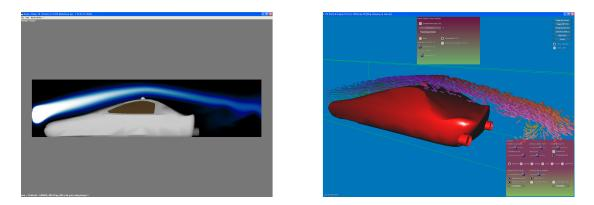
Figure 7.10: The left screenshot shows the design view in the "NavierStokes2D". The right screenshot depicts the same project in the particle engine; the flow is visualized using oriented point sprites (see Section 5.3.5).
