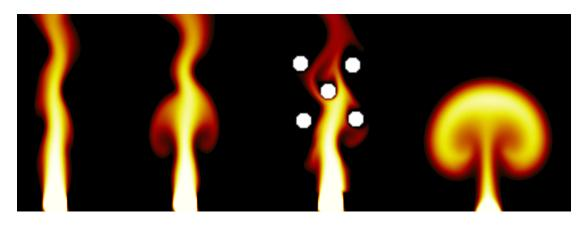
Figure 4.6: From left to right we show a simple inflow, the same flow with vorticity confinement enabled. The next image depicts a few obstacles placed in the flow while the rightmost picture shows a temperature driven inflow
