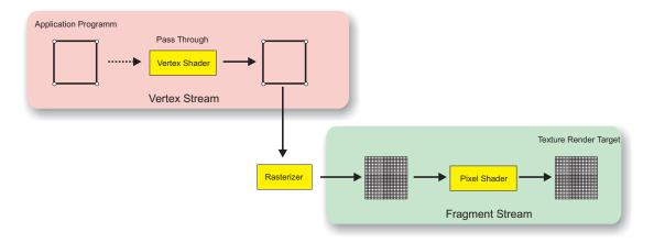
Figure 3.3: The basic setup of the rendering pipeline for a GPGPU computation. The computation is initiated by a single viewport-covering quadrilateral. This quadrilateral is converted by the rasterizer into a fragment stream. This stream in turn initiates the computation in the pixel shader.
