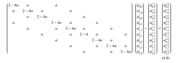
By using the GPU linear algebra framework these operations can be carried out with a single call to the m->MatrixVectorOp(CL\_SUB, currentSurface, lastSurface, nextSurface) method of the matrix class. In this call currentSurface and lastSurface are GPU vectors containing the grid values at time-step t and time-step t - 1. The result is written into the vector nextSurface. To initialize the matrix m with its five non-zero-diagonals C++ code in Listing 4.1 is used.
