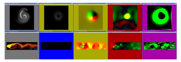
Figure 7.3: The screenshots show the five different render modes of the "NavierStokes2D" application. In the lower row from left to right, dye advection, the obstacle editor, the flow field view, the pressure distribution, and the rotation view are shown. The top row depicts the same modes for a different flow field. Instead of the obstacle editor, the second mode for the flow field view is shown; in this mode the vectors are drawn as little arrow glyphs instead of a color code.
