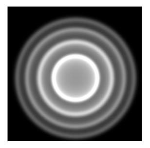
Figure 4.2: The image shows a quadrilateral textured with the solution vector of the water surface PDE. In this image the values in the vector texture are interpreted as grayscales.
