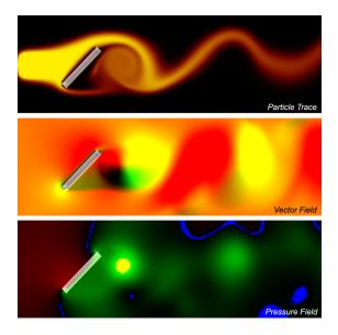
Figure 4.9: A vortex in the flow field, the vector field and the corresponding pressure field (red and green indicate high and low pressure regions, respectively).
