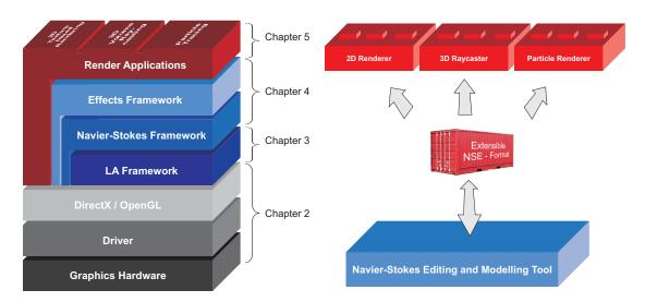
Figure 7.1: The blue and red blocks in left image show the software stack of modules developed in chapters 2 to 5 in this thesis. The gray blocks demote system and GPU vendor layers, blue blocks indicate the LA and simulation layers, and the red blocks finally contain the rendering applications. The right image depicts the horizontal data flow via the Navier-Stokes Equation container, which allows all applications to work on common data.
