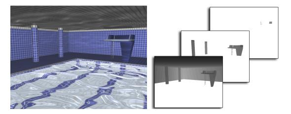
Figure 6.6: The caustics pool demo is shown on the left. In the right image the first three depth layers can be seen.
