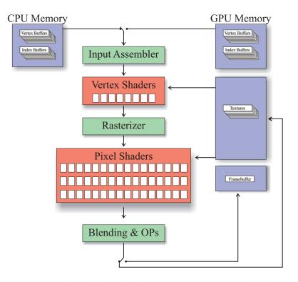
Figure 3.1: The figure shows the pipeline of a DirectX 9.0c GPU. Red boxes indicate programmable pipeline stages. Within these the white boxes show the number of pixel and vertex shader units for current GPUs, in this case an ATI Radeon X1900 [7].
