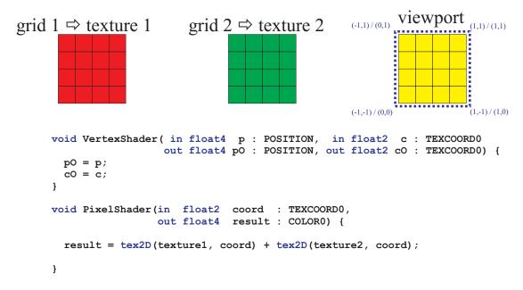
Figure 3.4: This Figure shows the setup of the rendering pipeline for the sum computation of two grids. The grids are stored in two textures, with a third texture bound to the viewport as render target. The dotted blue square around the viewport depicts the position and texture coordinates of the full-screen quad. Below the textures are the vertex and and pixel shaders in HLSL code.
