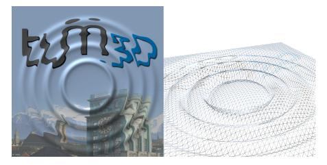
Figure 5.24: Rendering the height field of the shallow water equation in different modes. The left image shows the water surface with the refraction shader. In the right image the height field was used to displace a triangle grid.
