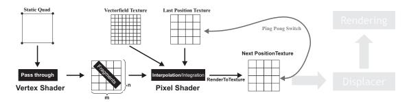
Figure 4.17: GPU Particle Advection. The black part of the image depicts the general GPGPU setup used for particle advection. The pixel shader takes as input the vector field and the current positions of the particles and computes the new advected positions. These positions can be used to drive a particle rendering engine (gray blocks, explained later in Section 5.3). In the next iteration the position textures are swapped and the advection process is repeated.
