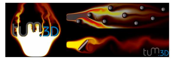
Figure 5.4: 2D texture-based rendering using dye advection
