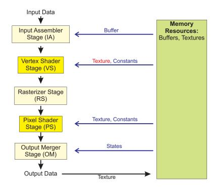
Figure 2.4: The Direct3D 9c Pipeline. Yellow boxes denote the two programmable stages. Note the red "texture" on the arrow to the vertex shader, this is one of the important additions to the pipeline by the Shader 3.0 API.
