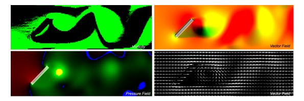
Figure 5.2: On the left side the vorticity, pressure distribution, and on the right side the flow field itself is shown. The bottom right image shows a particle-glyph based visualization of the same flow field, for comparison.
