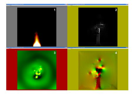
Figure 7.11: Flow design for the cigarette smoke demo. With a heat source on the bottom and pressure templates above the flame, a "pseudo-turbulent" fire flow is modeled. The four screenshots show the dye-advection view (1), the glyph-based flow view (2), the pressure view (3), and the color coded flow view (4).
