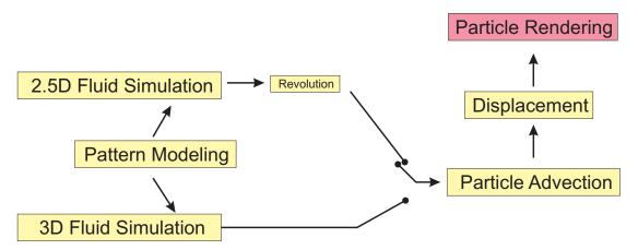
Figure 5.19: This image shows the principal interplay of some of the software components proposed so far. The combined components allow for the rendering of particle-based fluid effects such as the smoke in Figure 5.20.
