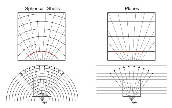
Figure 5.8: Different proxy geometries used in texture-based volume rendering. Note the non-uniform sampling (red) when rendering planes instead of spherical shells.
