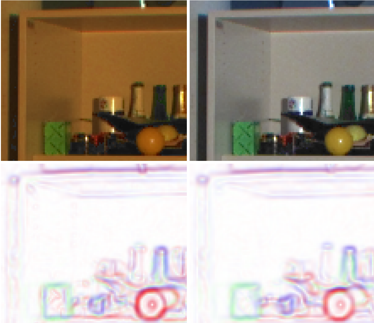
Figure 4.11: Influence of white balancing on demosaicing results. Left column: no white balancing is applied before demosaicing. Right column: white balancing (white patch algorithm explained in section 4.3) is applied before demosaicing. Top row: demosaicing results. Bottom row: m space gradients computed on the demosaiced images. These gradients allow a better visualisation of colour artifacts. Colour images are gamma corrected for better visualisation ( \gamma = 1.5 ). Gradients images are scaled between 0 and 255.
