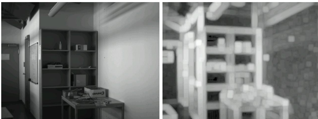
Figure 3.7: Grey value image and corresponding local standard deviation of CF estimated on a 15 \times 15 window. The grey value image is gamma corrected ( \gamma = 1.3 ). For better visualisation, the logarithm of the local standard deviation of CF is shown after normalisation between 0 and 255.
