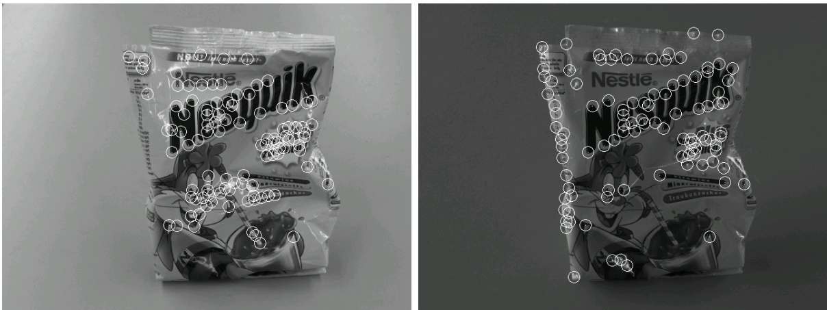
Figure 3.1: Detection example for the Harris detector with selection of the N best points ( N = 100 ). The images show the same scene under two different illuminations. 46.1% of the interest points of the left image are redetected in the right image. 51.6% of the interest points in the right image are false positives: they do not correspond to any interest points of the left image. Both images are gamma corrected for visualisation ( \gamma = 1.4 ).
