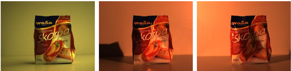
Figure 5.18: Three different illuminations for the test images of object 10. No white balancing is applied.
