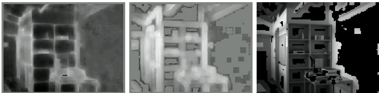
Figure 3.15: Results of the ISODATA algorithm on 25 \times 25 neighbourhoods ( L ) of \ln(|CF|) . The small neighbourhood S is 5 \times 5 wide. Left: low cluster mean \mu^{low} . Middle: high cluster mean \mu^{high} . Both images are scaled with the same parameters for visualisation. The areas with constant grey value are areas for which the high cluster contains no pixel. Right: detected textured area. Homogeneous areas are indicated in black. T_1 is set to 2.5 for the detection of textured areas with \mu^{high} - \mu^{low} > T_1 .
