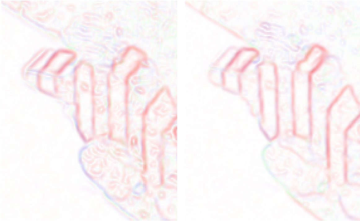
Figure 4.17: Influence of the preprocessing on the m space for a detail of the gradient images in fig. 4.16. Left: m space gradient with preprocessing as for HC-HD and with white balancing before demosaicing. Right: m space gradient with the preprocessing designed in section 4.6.
