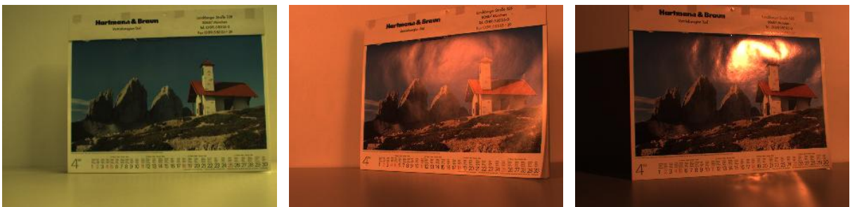
Figure 5.18: Three different illuminations for the test images of object 10. No white balancing is applied.
