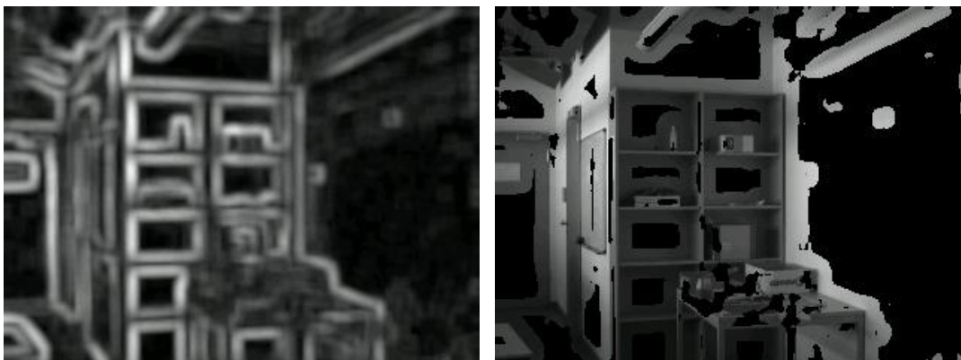
Figure 3.10: Detection of the textured areas by thresholding the local standard deviation of \ln(|CF|) estimated on a 21 \times 21 neighbourhood. Left: standard deviation normalised between 0 and 255. Right: detection result. Homogeneous areas are indicated in black. For visualisation, the grey values are gamma corrected ( \gamma = 1.4 ).
