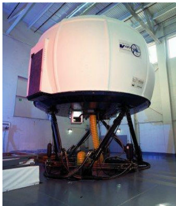
6 Freiheitsgrade, Standard-BWS • xyz-translatorisch • xyz-rotatorisch Ford, Safety and Research Development Department
