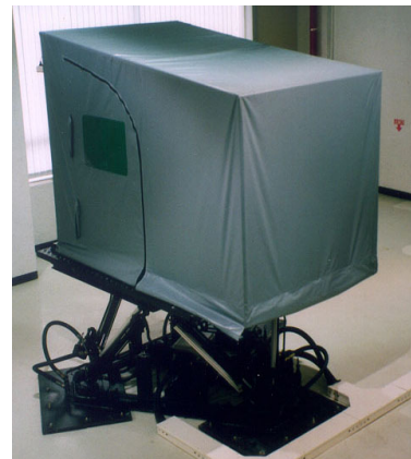
6 Freiheitsgrade Standard-BWS • xyz-translatorisch • xyz-rotatorisch Kookmin University, Mechanical and Automotive Engineering
