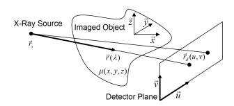
Figure A.1.: Scheme of X-Ray projection imaging
