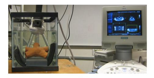
Figure B.2.: Clay phantom submerged in water
