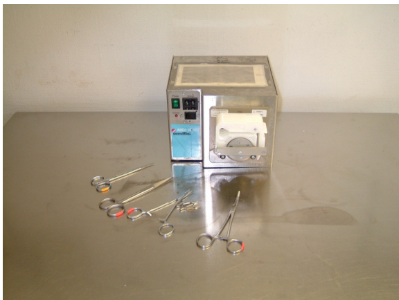
Abb.24 Perfusionspumpe: Regio Analog, Modell ISM 830 (Wertheim-Mondfeld).
