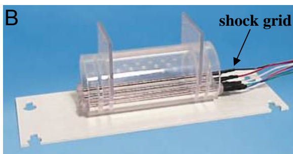
Fig 23 (A) Picture of the interior side of the sound-attenuating cubicle used for the Fear Potentiated Startle protocol. The major elements described in more details in the Materials and Methods session are indicated; (B) Higher magnified view of the plastic animal holder with the shock grid inside.
