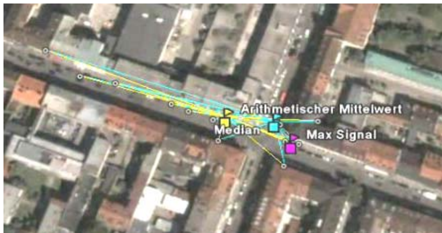
Figure D 3 Initialization examples showing Mean, Median and Point-of-Max. RSS calculations for a cluster prototype at particular GPS reference point instance
