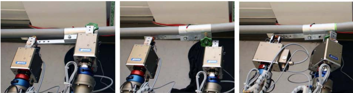
Figure 5.4: Used strategies of the participants. Left: horizontal orientation of clamp. Middle: vertical orientation of clamp, fixing of wheel by pushing against grooves. Right: vertical orientation of clamp, fixing of wheel by rotation
