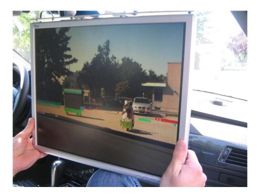
Figure 9.13: Snapshot of the See-Through TFT. One can see the superimposed sensor data on the garbage container and the Vespa scooter
