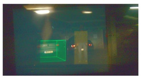
(b) The image has been taken in a basement garage and shows the detection results of the perception system (pedestrian: yellow box, vehicle: green box)
