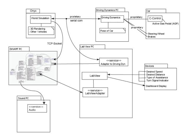
Figure 5.4: The Rapid Prototyping environment after the first modification step
