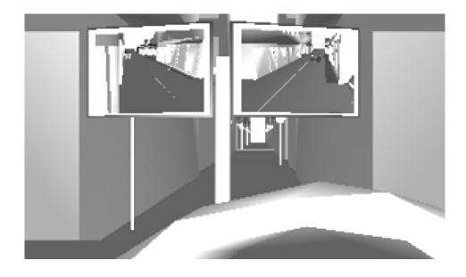
Figure 4.9: Virtual Side Mirror in the HUD showing the view to the left and right, thus reducing blind areas; courtesy of [57]
