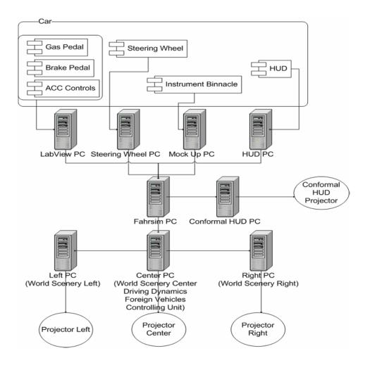
Figure 5.8: The Hardware Architecture of the new fixed-base Driving Simulator at the Chair of Ergonomics
