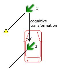
Figure 8.7: Sketch for the cognitive transformation of the pointing scheme. Arrow 1 shows the real position and arrow 2 the transformed one
