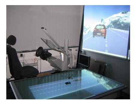
Figure 6.2: The system setup: The table-top environment in a tracking volume, where the tangible car can be moved around. The system is connected to a driving simulator
