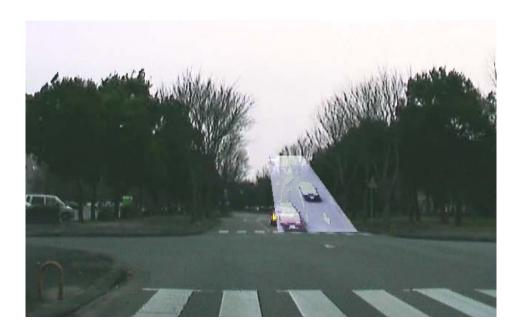
Figure 4.10: Virtual Slope Visualization in the HUD showing the opposite lane at an intersection tilted up so that occluded vehicles become visible; courtesy of [146]
