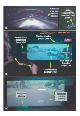
Figure 4.2: Display Modes of Holistic User-centric System: (a) in a constant single location, (b) at or near the driver's line of sight, and (c) on top of obstacles as perceived by the driver; courtesy of [161]
