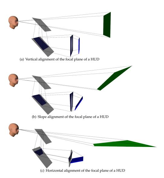
Figure 3.5: Different Alignments of Focal Planes to the line of sight of the Driver generated through different HUD Setups. Tilting the Display (blue) tilts the Focal Plane (green). Next to the Display is a Lens to stretch the Focal Distance. A Mirror (lower left) eases the Setup and the Windshield (upper left) combines the Views
