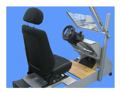
Figure 6.4: The driver's cockpit is build on an aluminum frame and has the same relationships as a common driver's cockpit (distances and sitting height)
