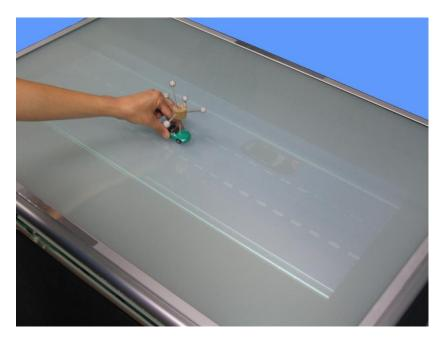
Figure 6.8: The tangible miniature car can be controlled from every side of the table allowing test participants to get into their preferred maneuvering position
