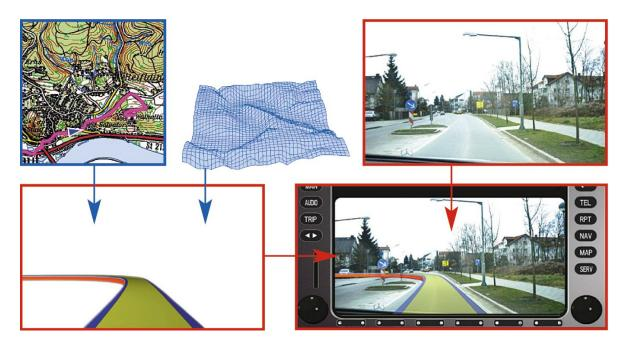
Figure 4.3: GPS information and 3D topography information are used to compute a 3D model of a navigation path which is superimposed on the in-car display of a navigation system; courtesy of [139]
