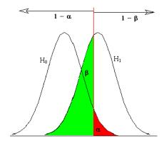
Figure 2.9: Sketch explaining distribution and probability of an  $\alpha$ - and  $\beta$ -error around a mean value
