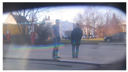
(a) The image shows sensor data from the automotive laser scanner. The persons' legs and the curbstone can be seen superimposed with sensor data.
