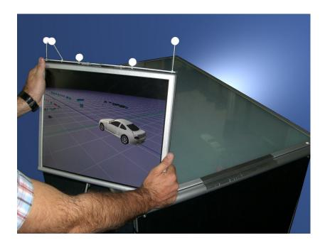
Figure 9.8: The portable TFT held into the tracking volume at the laboratory visualizes the virtual test vehicle and the perceived laser scanner data. The same scene is rendered from a birds-eye view on the back-projection workbench below
