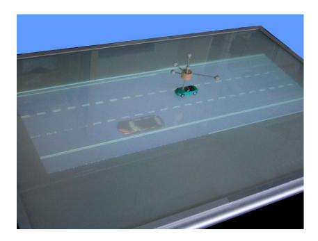
Figure 6.5: The table-top environment is built with a back-projection workbench and is placed in an infrared tracking volume
