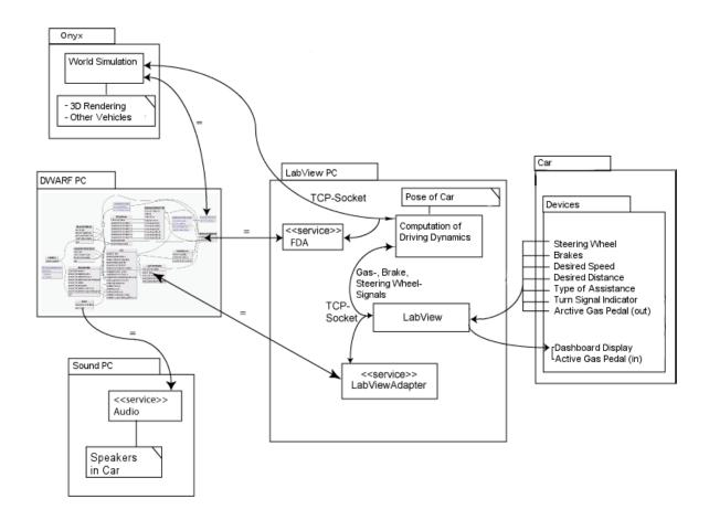
Figure 5.6: The implementation of the final rapid prototyping environment in the first driving simulator
