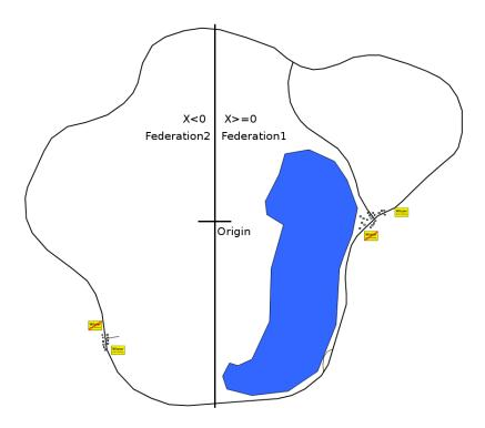
Figure 6.17: The road course of the driving simulator. *Federation1* manages the positive side of the X-Axis, *Federation2* the negative
