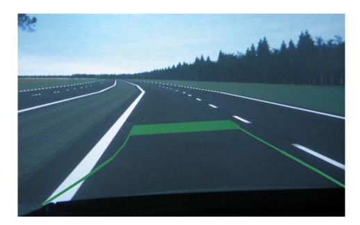
Figure 7.5: A screenshot showing the braking bar and the drive-path in a light left curve. One can see the car actually is slightly too far to the left and starts the left curve too early
