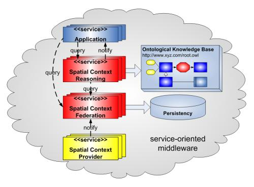
Figure 6.13: Architectural Overview of SCORE: Trackers define Spatial Context Providers that update Spatial Context Federation components. These are queried by components for Spatial Context Reasoning. ADAS Applications on top specify the user interface for the driver
