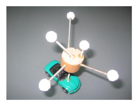
Figure 6.1: The tangible miniature car: A small green BMW Z3 series in a scale of 1:100 with attached 6 dof marker tree.
