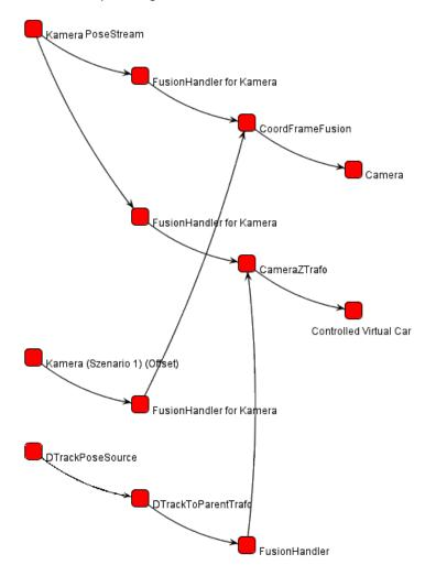
Figure 6.10: The part of the dataflow network responsible for the base speed of the tangible car
