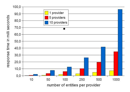
Figure 6.19: Overall response times of the entity histories of the access interface method of the federation service (n-to-n query)
