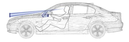
Figure 2.6: The principle of a HUD, a bright display behind the dashboard generates the image that is mirrored into the windshield and appears in distance of the front bumper (courtesy of BMW)
