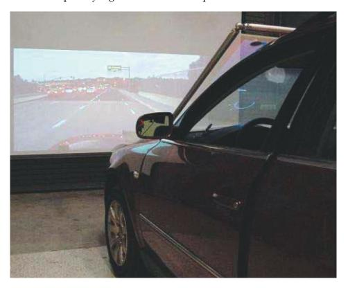
Figure 4.1: Full Windshield Head-Up Display in Driving Simulator; courtesy of [161]
