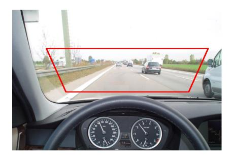
Figure 2.7: A Driver's Frontal View with outlined minimal Area for a Large Scale HUD
