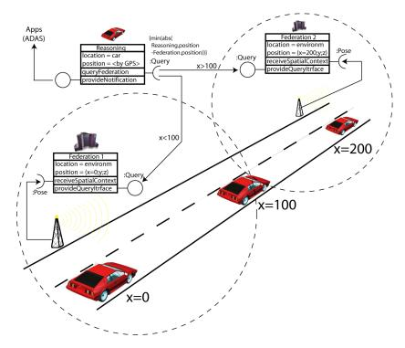
Figure 6.16: Sketch of dynamic reconnection of car internal reasoning service between two federation service sectors as car moves along X-axis
