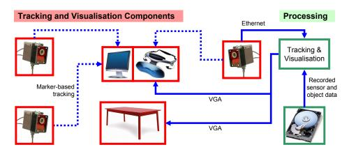
Figure 9.1: Overview of Hardware Components of the Lab Setup
