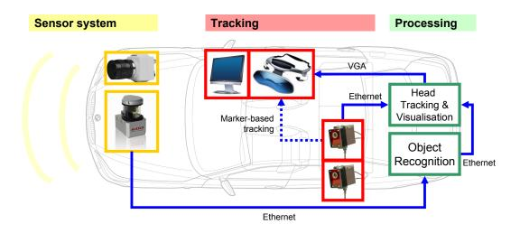
Figure 9.3: Overview of the hardware components, the communication channels and the rough respective installation locations in the test vehicle
