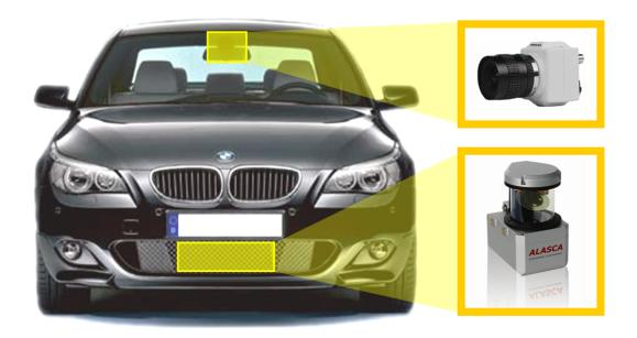
Figure 9.2: Mounting points of the two perception sensors. The automotive video camera is located behind the windshield and the laser scanner beneath the license plate
