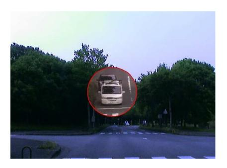
Figure 4.8: Virtual Back Mirror floating in the HUD showing the correctly transformed view of a fixed camera on the street; courtesy of [113]
