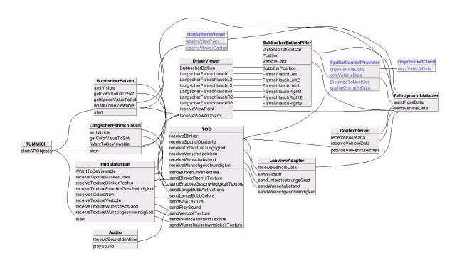
Figure 5.5: Screenshot of the DWARF network mainly running on the computer dedicated to DWARF. The boxes are the service components and the connecting lines show the data flow between the components.
