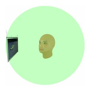
Figure 3.2: The *Sphere of Vision* adapting to a tracked LCD display: The nearer the display gets to the head, the smaller the sphere but the wider the field of view
