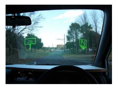
Figure 4.7: Navigation Information through navigation flags and direction signs; courtesy of [131]
