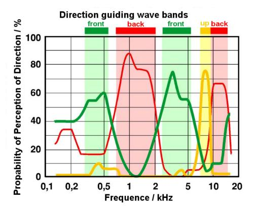
Figure 8.13: Relationship between acoustic frequency and human understanding of relative direction; adapted from [26]
