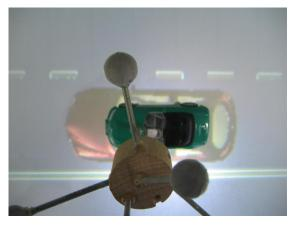
(b) Photography of a scaling with unequal size. The virtual car model is about 1.6 times the size of the miniature car
