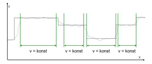
Figure 7.6: A sketch that illustrates the four intervals, where a constant speed should be maintained. The four intervals are constrained by increases or decreases of the allowed speed
