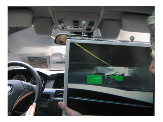
Figure 9.12: The TFT held into the tracking volume while driving. One can see the green augmentation of the detected vehicles
