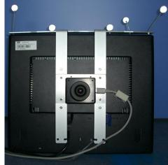
(a) HMD (Sony Glasstron PLM-S700) used for (b) Backside of the 19" TFT video see-through visualization worn by an artificial head display with an attached FireWire camera at the center
