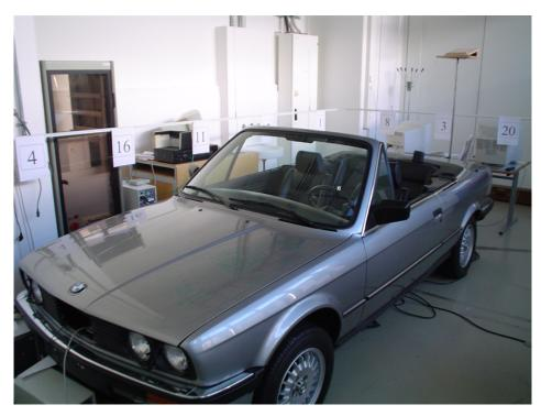
Figure 8.3: Driving Simulator surrounded by Numbered Sheets at Eye Level
