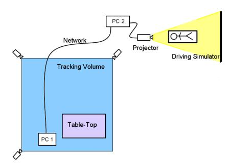
Figure 6.3: The Miniature Car Table-Top Environment – Sketch of the Setup
