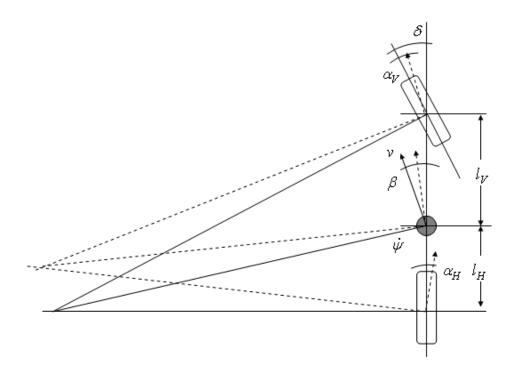
Figure 7.4: Principle of Single Track Driving Dynamics Model. A two wheeled vehicle follows a circle section
