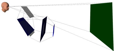
(b) Setup using the same optical elements but placing the focal plane in large distance: the field of view became wider
