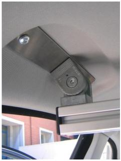
(a) Overview of Mount for the Tracking Sys- (b) Left side Handhold Mount for Tracking System
