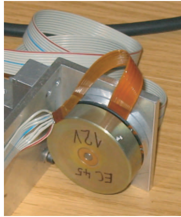
Figure A.3: Synchronous motor.
