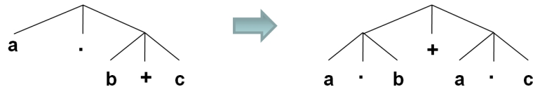
Figure 5.16: Tree-based representation of the distributive law as structure transformation applied to operator trees .
