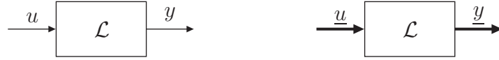
Fig. 2.1: Block diagram representation of signals and LTI-systems: Thick signal arrows (block diagram on the right) represent a vector of signals, i.e. \underline{u}(t) = [u_1(t) \dots u_r(t)] , e.g.. In this case, the LTI-block \mathcal{L} represents r independent SISO LTI-systems so that [y_1(t) \dots y_r(t)]^T = \mathcal{L}(\underline{u}(t)) := [\mathcal{L}(u_1(t)) \dots \mathcal{L}(u_r(t))]^T .
