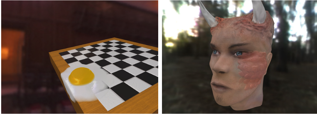
Figure 6.16: Results of the proposed displacement method (I). Left: Demonstrating that using rotations to propagate directions does not fail at acute angles. Right: Augmenting a game character to obtain a highly detailed and naturally looking appearance. The displacement was given a light red hue in order to make it discernible. Devil Head mesh courtesy of Thomas Heinrich.
