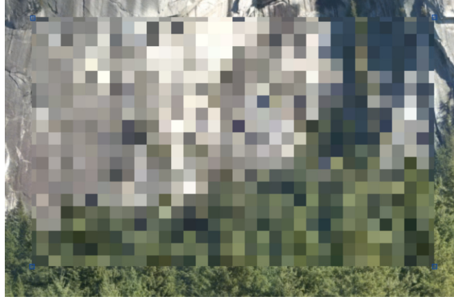
Figure 7.9: A Log-Reduce filter to compute the maximum. The maximum of 128^2 pixel blocks is obtained in 7 dyadic steps. Data courtesy of Johannes Kopf and Prof. Dr. Oliver Deussen, University of Konstanz, Germany.
