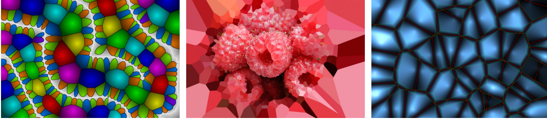
Figure 7.12: Different Voronoi diagrams. From left to right: A generalized Voronoi diagram using points and curves as sites, an artistic Voronoi-based mosaicking filter using Gaussian-distributed sites, and a Voronoi diagram consisting of first- (red lines) and second-order (green lines) neighbor regions (please refer to the electronic version). Each image has a resolution of 1600 \times 1200 and was generated completely on a GPU. The two left images took less than 22 ms, the rightmost image took less than 31 ms.
