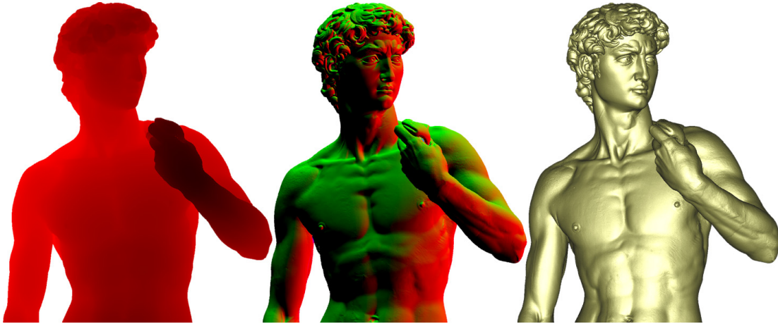
Figure 3.16: The three passes needed for our deferred shading approach. Left: The first pass generates a depth image. Middle: During the second pass the depth of incoming fragments is compared to the depth image obtained in the first pass. Fragments with a depth further than \varepsilon away from the respective depth of the first pass are discarded. The remaining fragments are blended in order to accumulate their properties. Right: In the third, purely image based pass the attributes accumulated in the second pass are used to illuminate the final image. Data courtesy of the Digital Michelangelo Project.
