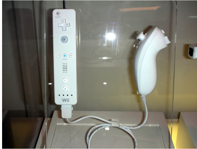
Figure 7.5: Photograph of a WiiMote with Nunchuk. The WiiMote (left) is used in for user interaction. It is a low-cost device that is tracked by means of IR-based triangulation and accelerometers. The Nunchuk (right) can be disconnected from the WiiMote and is not used in this work. The image is under the Wikimedia Commons licence.
