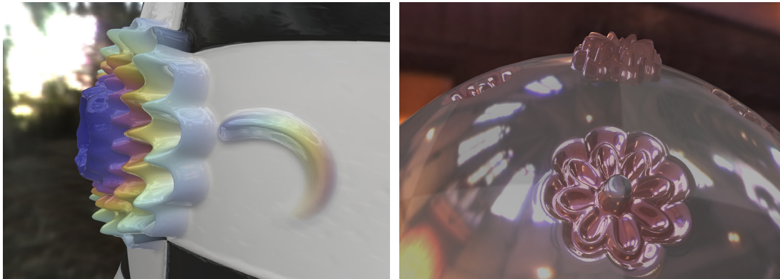
Figure 6.19: Results of the proposed displacement method (IV). Left: Our method is capable of smooth transitions between base surface and displaced geometry. This is achieved simply by providing height fields with a smooth fall-off to their zero-level. Furthermore, appearance properties such as tangent frames, colors, and texture coordinates can be propagated from the base mesh. Right: Positive and negative displacements at the same time can be handled by our method.
