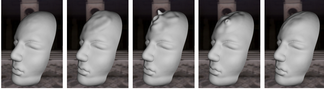
Figure 6.18: Results of the proposed displacement method (III). A water simulation on a circular domain is used to animate the displacement field. The simulation was pre-computed on a 256^2 grid and has 319 time steps. We achieve a rendering performance of over 140 frames per second on a 1600 \times 1200 view port. Base mesh courtesy of Aim @ Shape.
