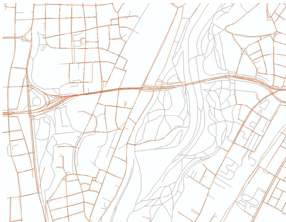
Figure 6.17 Differences of the road networks between NAVTEQ (orange) and ATKIS (grey)
