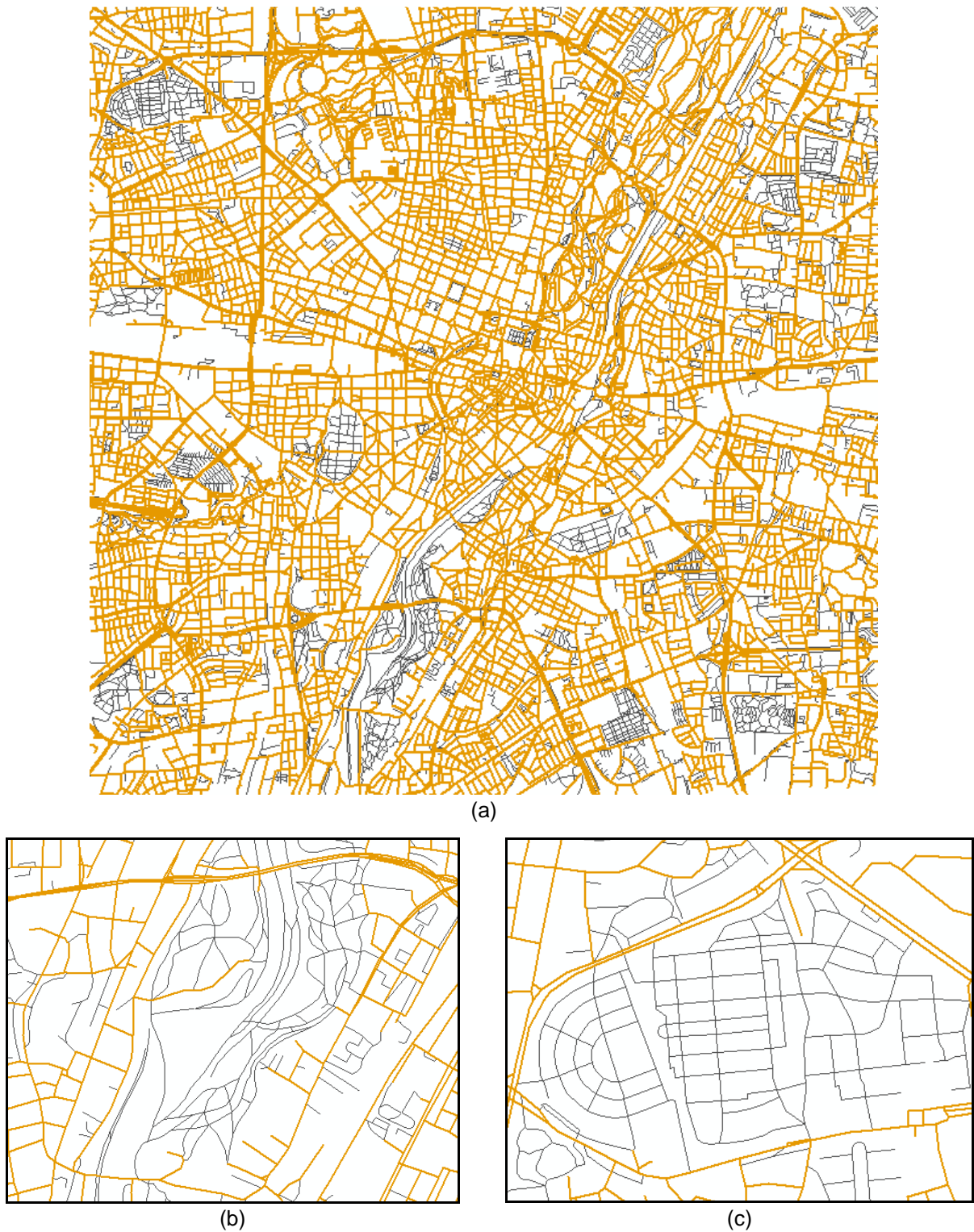
Figure 6.24 An example of the conflated road network in a built-up area ( 10 \times 10 \text{ km}^2 , Munich, Germany)
