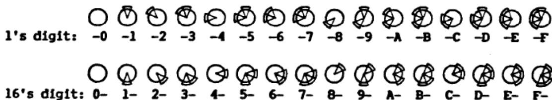
Figure 2.5 Hexadecimal and sector patterns for spider function (Saalfeld 1988)
