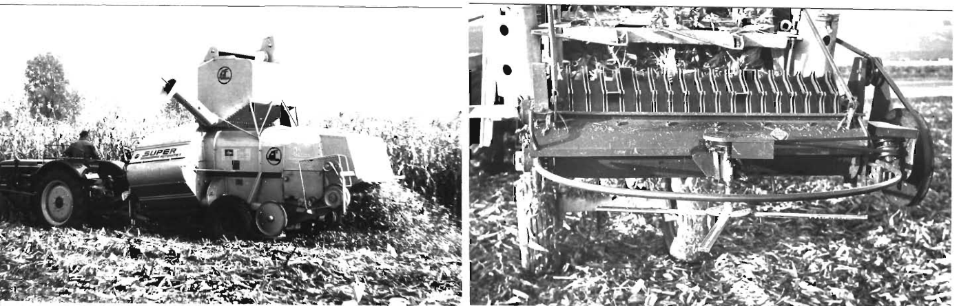
Abb. 40: Anbau-Strohhäcksler (links System Claas, rechts System Meyer)
