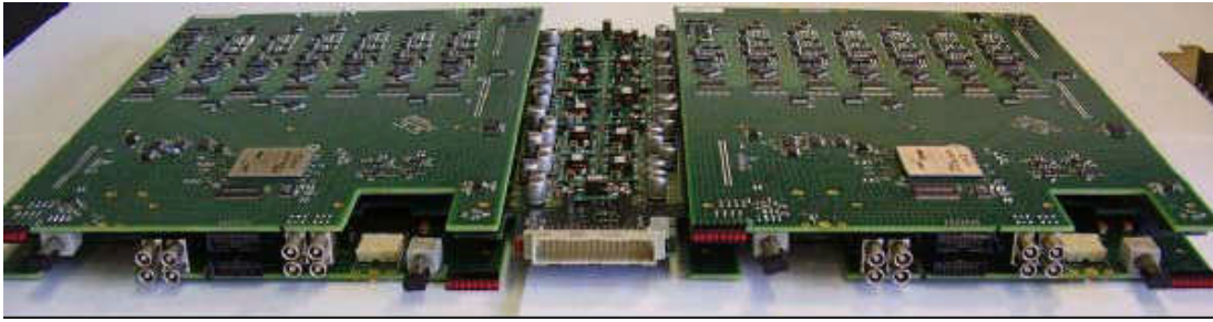
Figure F.2: The electronics board of one AGATA digitizer, without the housing. In the back part the sampling ADC's, one for each of the 38 channels, are visible. The FPGA's used for synchronizing the channels and formatting the data for the optical links are in the front of this picture. The figure was taken from (Simpson et al., 2008).
