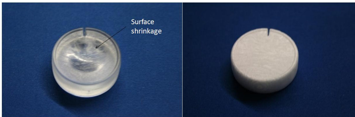
Fig. 5.29: Molded parts from compact and foaming injection molding by mold B Left is the compact molded part by TPU, right is foamed part. The left sample showed a clear surface shrinkage, which was not possible to solve by compact injection molding, but the right foamed sample showed no surface shrinkage.
