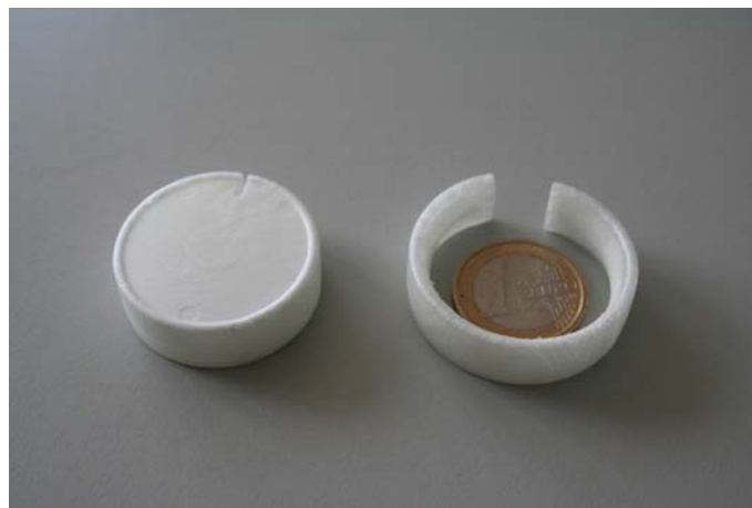
Fig. 6.1: The implant (left) and the ring after removal of the core (right)
