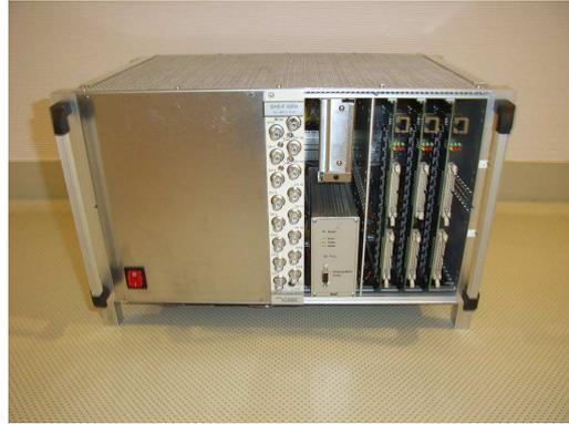
**Figure 6.13:** Electronic system for the MADPET-I lab course, including all power supplies (low-voltage, high-voltage), rotating table control and three SADC modules with USB readout (*right*). [Sch09]
