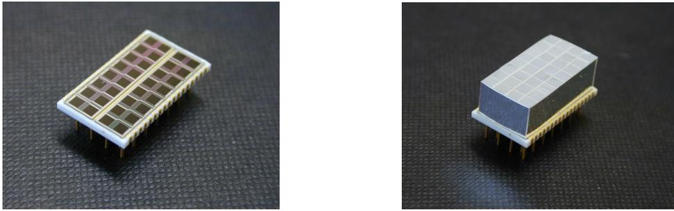
**Figure 3.3:** Hamamatsu Photonics S8550  $8 \times 4$  APD array (left) and APD array with mounted scintillator crystals for the first detector layer (right).
