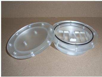
**Figure 6.16:** Sample source for the lab course with the TUM logo as active region. The source is milled from plexiglas and can be filled with  $^{18}\text{F}$ -FDG. [Sch09]
