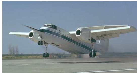
Figure 14. de Havilland C-8A Augmentor Wing research aircraft (NASA 2009)
