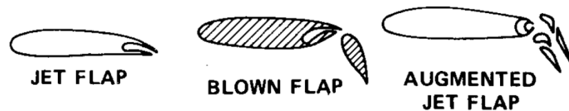
Figure 11. Examples for Internally Blown Flaps (Englar and Hemmerly 1981)
