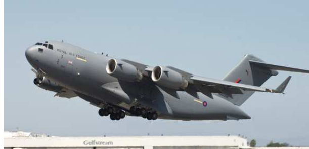
Figure 10. Boeing C-17 military transport aircraft with EBF (Boeing 2009a)
