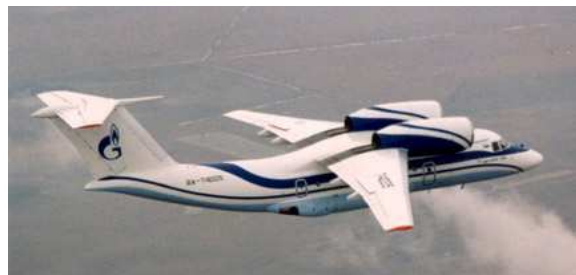
Figure 8. Antonov AN-72/74 transport aircraft with USB (Antonov 2004)
