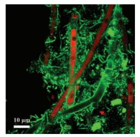
FIG. 2. Probe-related signals after FISH applied on a single-granule microsection of 30-µm thickness. The image shows fungal filaments colonized by bacteria in a granule developed in synthetic wastewater. Probe-related signals are recorded by CLSM after FISH with the *Bacteria*-specific mix of the EUB338 probes (fluorescein-labeled; green) and the *Eukarya*-specific probe EUK516.
