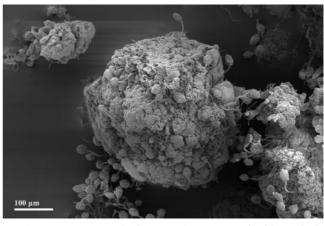
FIG. 6. Mature granule from an SBR operated with synthetic wastewater. The granule is spherical in shape and consists of bacteria and extracellular polymeric substances. It is colonized with many stalked ciliates of the subclass Peritrichia. SEM.
