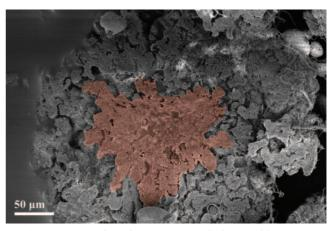
FIG. 8. Cross-section of a mature granule from malthouse wastewater. The dense core zone containing bacteria and possibly dead cell debris is recolored in red. The loose-structured fringe zone (gray) containing bacteria and ciliates encases the core zone. SEM.
