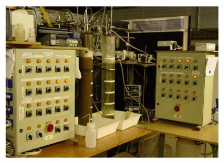
**Fig. 2:** Lab-scale SBR system with fully automated timers, used in this study. Left SBR filled with aerobic sludge granules and malthouse wastewater during aeration phase.
