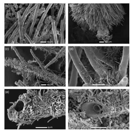
**Fig. 1.** Scanning electron micrographs of biofilm samples from SBR1 (malthouse wastewater; a, b) and SBR2 (artificial wastewater; c, d, e, f). Fungal filaments (hyphae) are implemented in the granule structure (a), with hyphae tips protruding from the granule surface (b). Hyphae are densely covered with rod-shaped bacterial cells both on the surface (c, d) and within the granule (e, f; visualized after cryo-fracture treatment).
