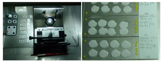
Fig. 7: Sectioning of granular biofilms. Granules were embedded after a fixation procedure in frozen section medium and cut into 25-30  $\mu$ m slices with a cryotome (left). Slices placed on gelatine-coated slides shortly before heat fixation (right).
