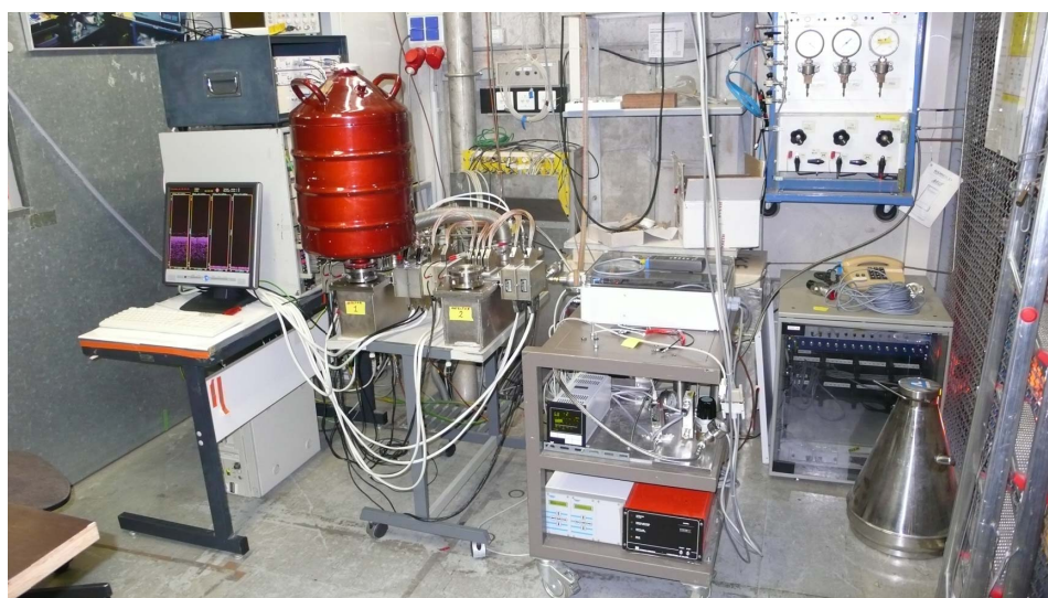
Figure 2.16: Photograph of the experimental setup: 2 COMPACT detectors with related electronics, and the gas control system.
