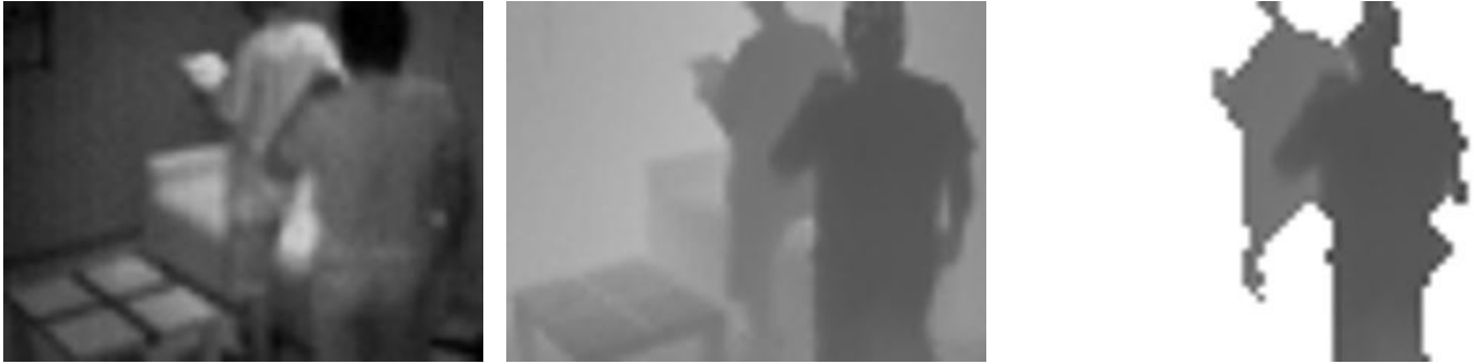
Fig. 1. 2 Persons approaching a sofa in a smart room. From left to right: NIR image of the scene with texture information, the aligned range image, and the segmented foreground region
