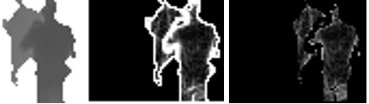
Fig. 5. From left to right: The segmented foreground region, the detected depth gradients, two foreground blobs after thresholding.
