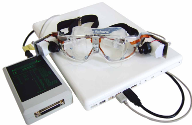
Fig. 2. EyeSeeCam head-mounted mobile eye tracking system.
