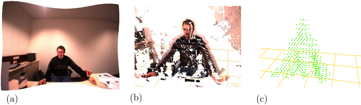
Fig. 3.4: Example of the Segmentation Process: (a) Image with detected skin parts as start point for the segmentation process. This image has been obtained by a stereo camera with a high aperture and has already been rectified. (b) shows the three-dimensional reconstruction of the scene using a stereo matching algorithm and (c) the detected segments in the scene.
