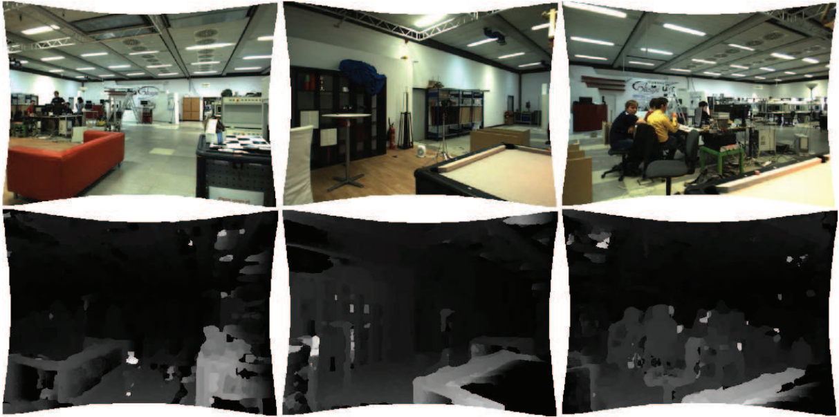
Fig. 3.14: Result of the stereo processing system. The upper row shows the left image from the stereo camera and the lower row shows the resulting disparity map. Points with a low confidence are indicated with black color.
