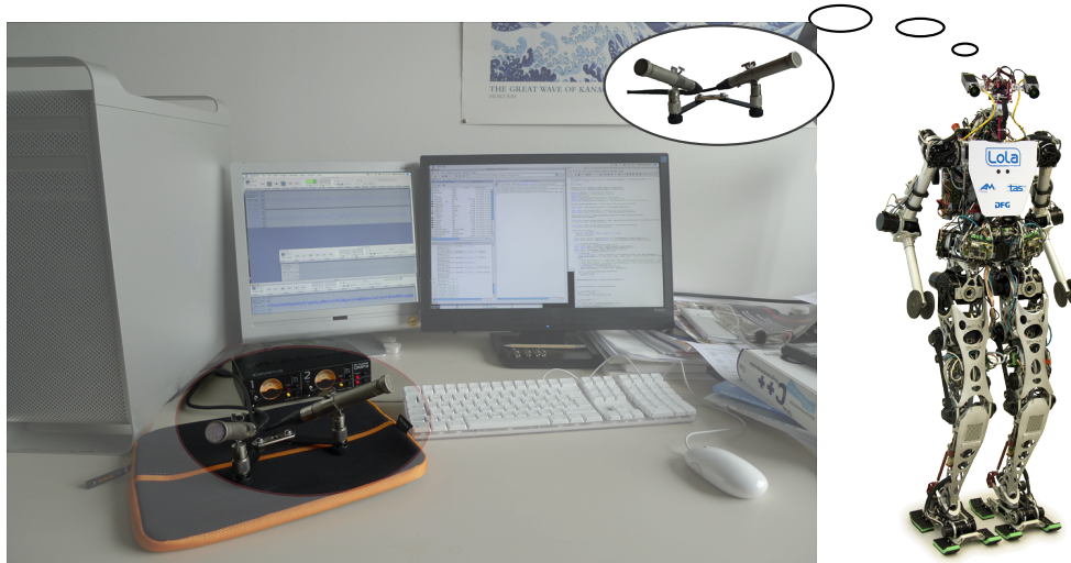
Figure 2.7: Experimental setup and future application. A pair of Oktava MK 012-01 microphones is used to record test sounds in a natural echoic environment, our office. The goal is to make our framework for echo suppression suitable for real-time processing in a multisensory robotic system, LOLA. Picture of LOLA by courtesy of the Institute of Applied Mechanics, TUM.
