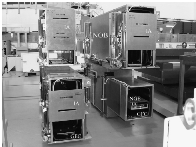
Fig. 4. View of neutron optical bodies (NOB) ready for being mounted into the beam guide chamber (NGE, UC and LC: neutron guide element and its upper (UC) or lower channel (LC); GFC: guide field coil; IA: interim aperture).
