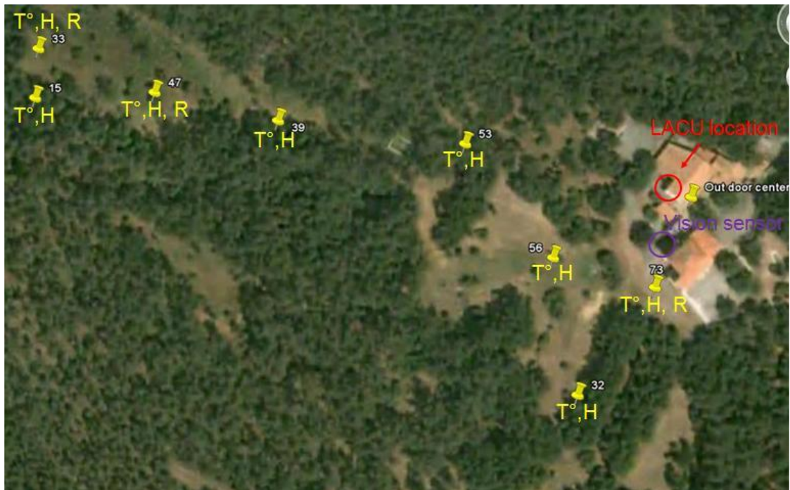
Figure 4-11 : Selected area and SCIER deployment -T: Temperature Sensor, H: Humidity Sensor- (Priggouris, et al., 2009)
