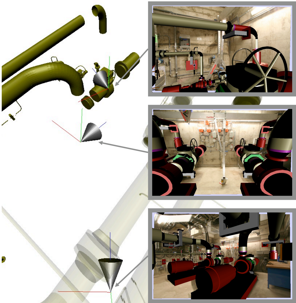
Figure 5.10: Example of a zoom in/out motion ; on the bottom with the most outer view and on the top the most inner view, the local geometrical relation is visible in the 3D scene; see that the viewpoints' directions do not need to be aligned.
