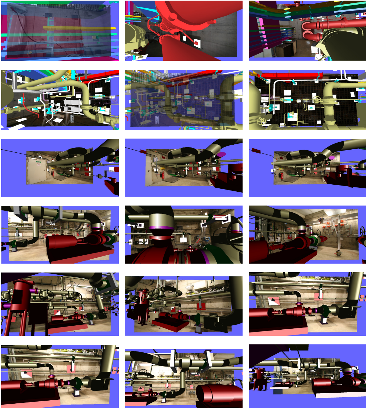
Figure 5.11: Example of left/right navigation The user can request a new view point that the presented algorithm estimates based on the focus of the current view. The left (resp. right) images corresponds to a requested view point from the center images to the left (resp. right).
