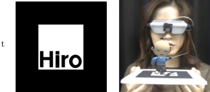
Figure 2.1: ARToolKit Markers : on the left the well-known “Hiro” tag and on the right a demonstration of ARToolKit to find the transformation between the marker and the user’s HMD. Courtesy of http://www.hitl.washington.edu/artoolkit/ .
