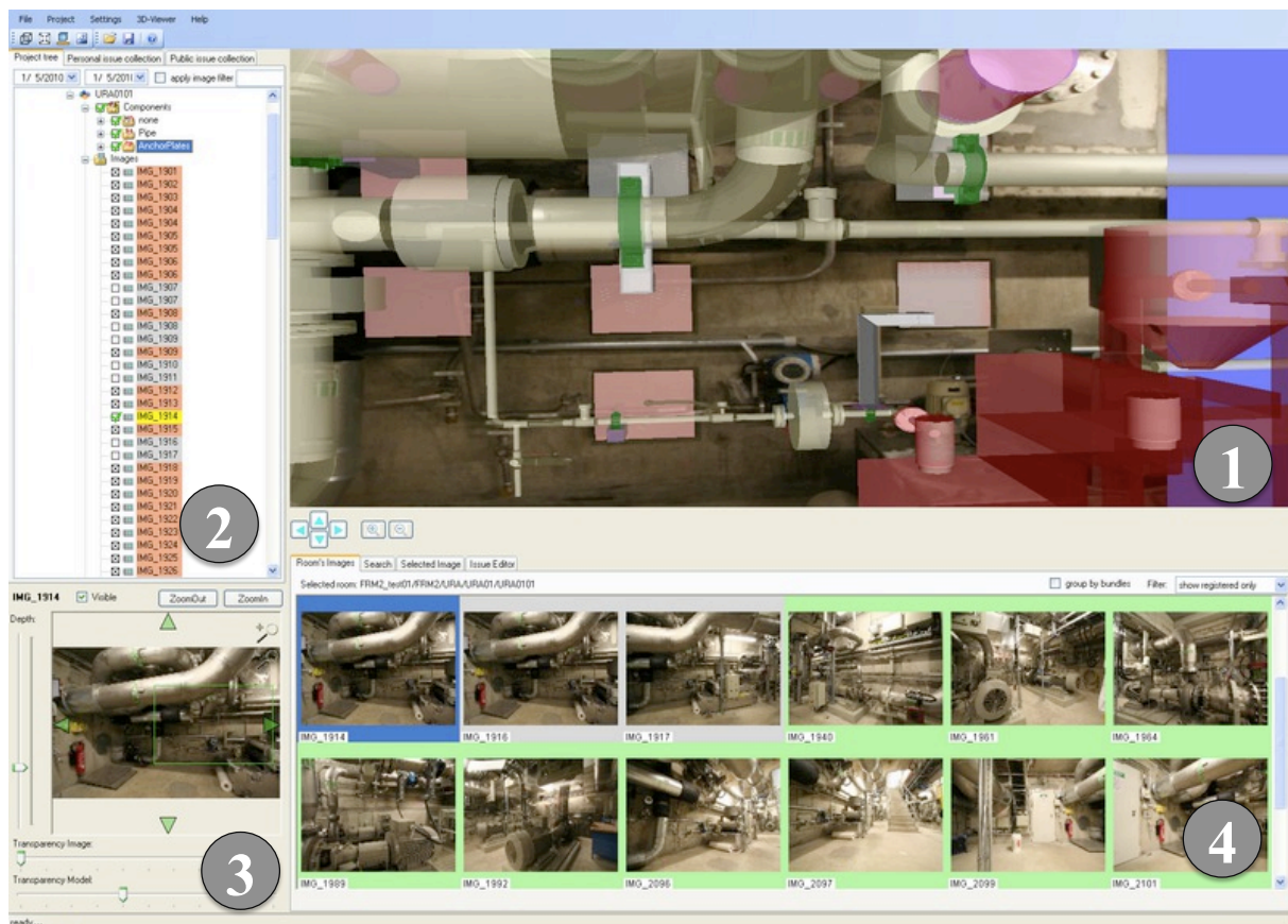
Figure 4.1: VID Main Graphical User Interface: (1) the 3D renderer that displays models and image, (2) the custom tree-view that gives access to the hierarchy of the project (3) the zoom and pan interface that command the virtual camera motion in a mixed view (4) the thumbnail browser that can display set of images based on a user-specified criteria.
