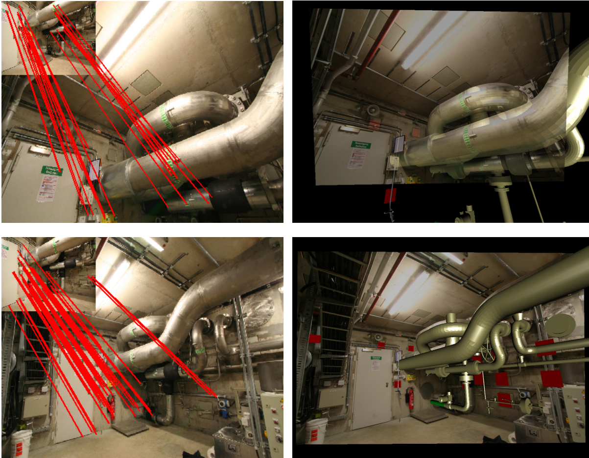
Figure 8.9: Hybrid Methods Applied to Images from an Industrial Compound: the left hand graphics represents the corresponding pair of points corrected using our method, the upper snapshot is the original keyframe; the right hand images display the resulting augmentation displayed in VID.
