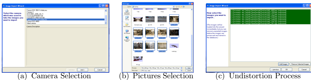
Figure B.4: Picture Importation GUI . The user is guided through a wizard to import newly acquired pictures. First, he selects the camera used, then the images from the disk, which are then automatically distorted. The new undistorted images are stored in the database.
