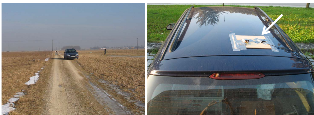
Figure 5.6: Experimental setup. The white arrow points to the patch antenna of the evaluation kit.
