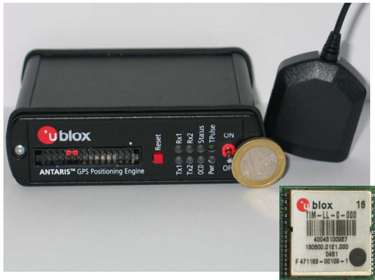
(a) Ublox evaluation kit with TIM-LL receiver module
