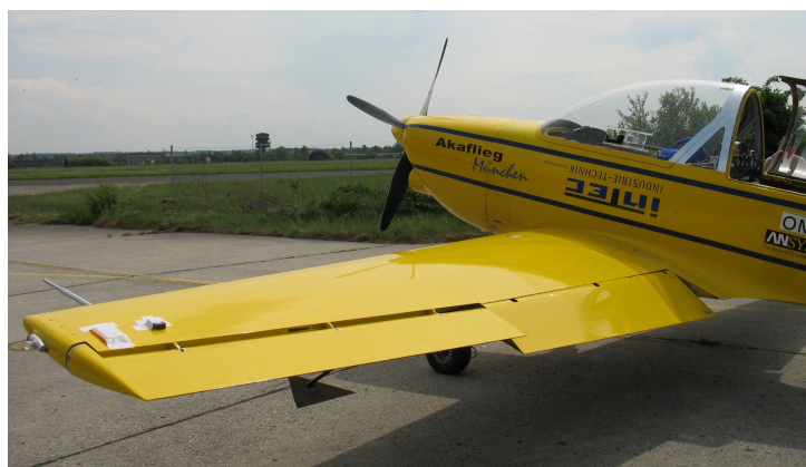
Figure 5.8: MÜ 30 “Schlacro” with the miniaturized receiver and data logger GiPSy mounted at the very outside of the wing
