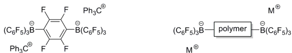
Figure 4.1. Structure of the trityl bisborate dianion (left), [9] potential polymeric bisborate dianion salts (right).
