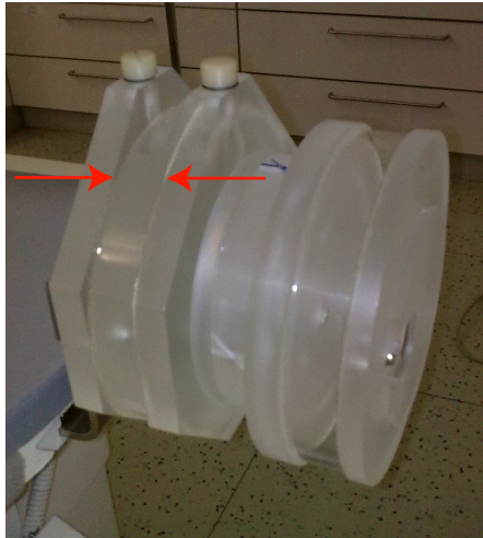
Figure 3.6: Standard Siemens phantom. The water region with a diameter of 20 cm and a height of 3 cm is marked by arrows.
