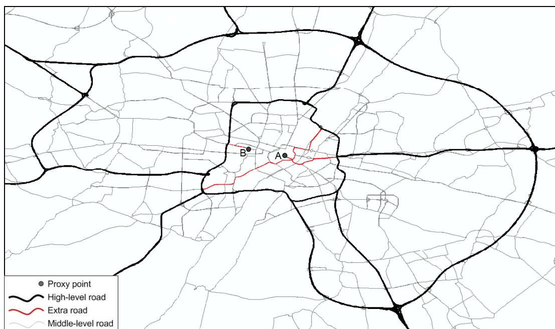
Figure 5.14 Selecting artifacts caused by proxy points in the road network for Munich
