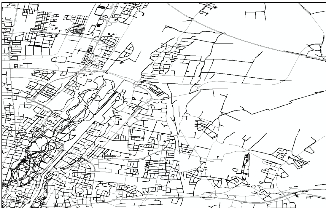
Figure 5.2 Omitted low-class roads (in bold) in the northeast of Munich (FRC=7,8 or N2C=5,6)
