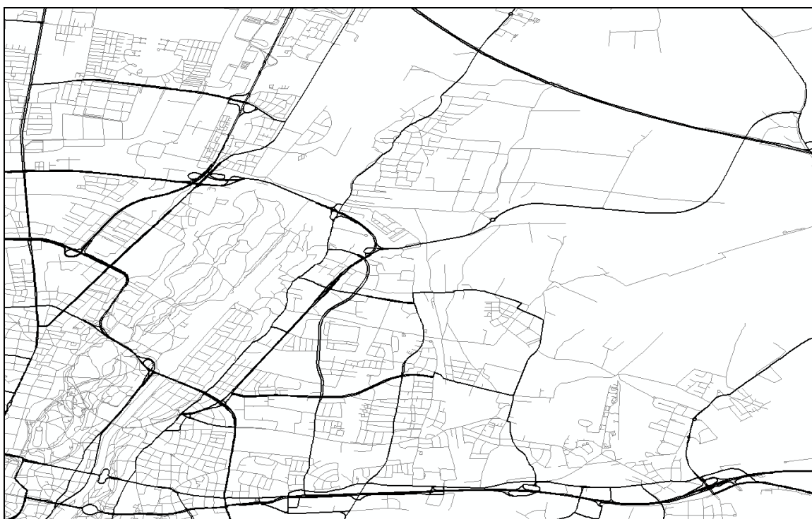
Figure 5.3 Selected high-class roads (in bold) in the northeast of Munich (FRC=0,1,2,3 or N2C=0,1,2,3 or NBC=1,2,4,5,6)
