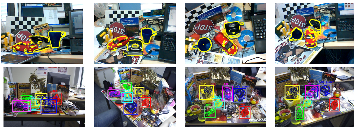
Figure 3.1: DOT Overview. Our templates can detect non-textured objects over little cluttered background in real-time without relying on feature point detection. Adding new objects is fast and easy, as it can be done online without the need for an initial training set. Only a few templates are required to cover all appearances of the objects.
