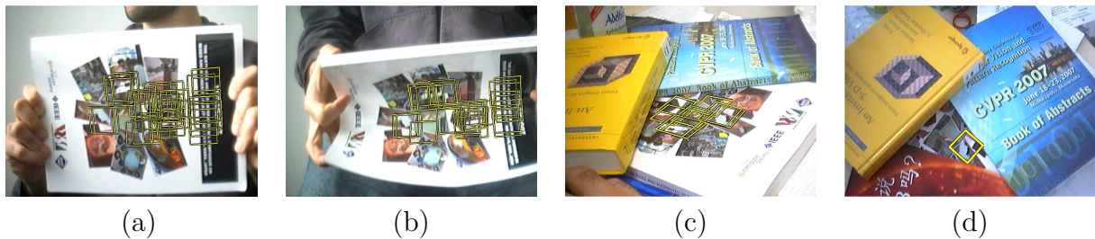
Figure 2.18: Robustness of LEOPAR to deformation and occlusion. (a) Patches detected on the book in a frontal view. (b) Most of these patches are detected even under a strong deformation. (c) The book is half occluded but some patches can still be extracted. (d) The book is almost completely hidden but one patch is still correctly extracted. No outliers were produced.
