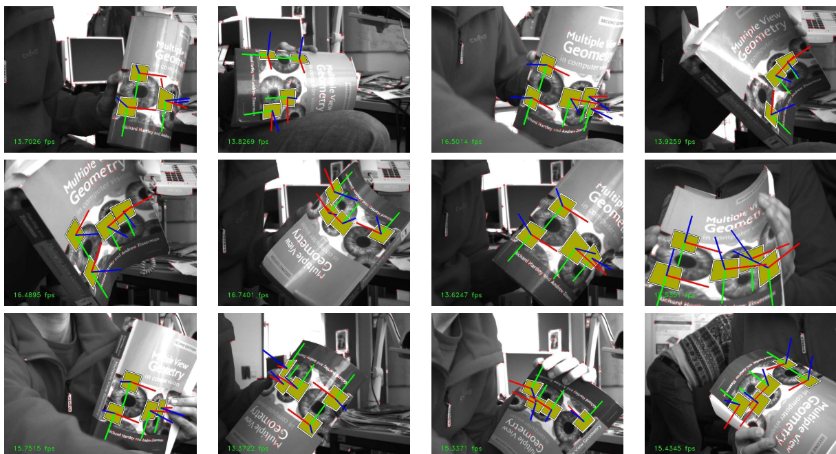
Figure 2.25: Application to a deformable object with GEPARD. We can retrieve an accurate pose even under large deformations. While it is not done here, such cues would be very useful to constrain the 3D surface estimation.
