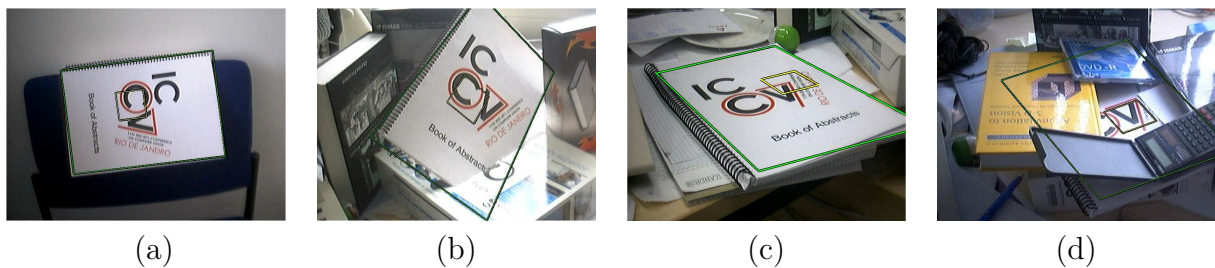
Figure 2.19: Accuracy of LEOPAR of the retrieved transformation. For each of these images, we draw the borders of the book estimated from a single patch. This is made possible by the fact we estimate a full perspective transform instead of only an affine one.
