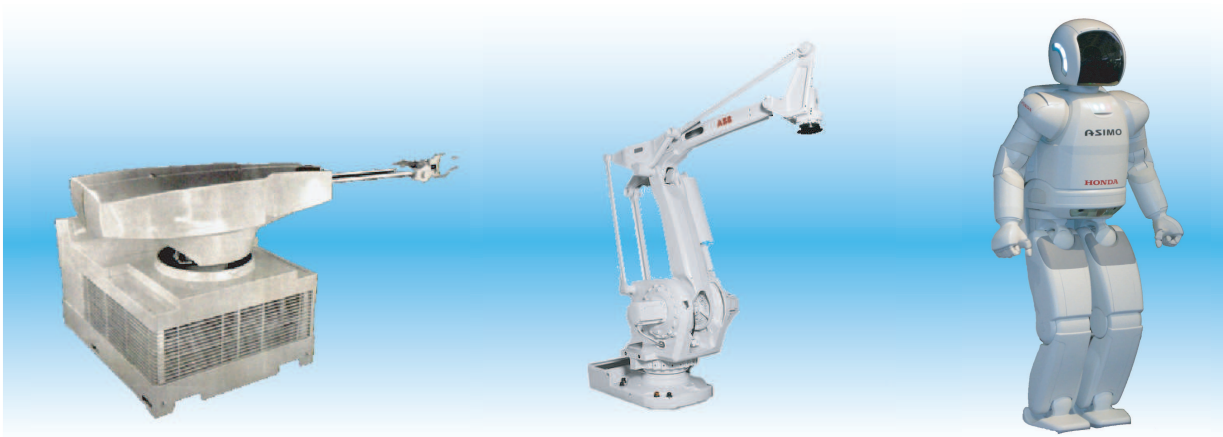
Fig. 1.1: The first industrial robot Unimate (left), the six DOF industrial robot IRB 260 from ABB (middle) and Honda’s humanoid robot Asimo (right).
