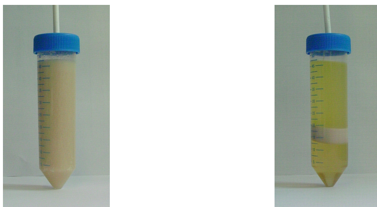
Figure 8.3: Emulsion before (left) and after (right) the phase separation by centrifugation. The centrifugation permits to completely separate the emulsion into its three composing phases: the aqueous phase (top phase), the cells (middle phase) and the ionic liquid (bottom phase).
