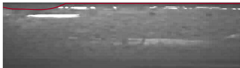
Figure 5.20: Air cavity at the top of a slug - v_f = 7.5 m/s
