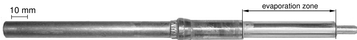
Figure 5.1: Heat pipe used as a corrosion probe for the iron loss tests
