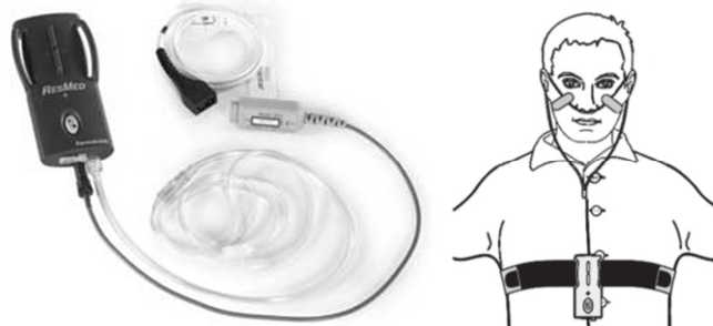
Figure 3.6: ApneaLink single-channel (nasal pressure measurement) screening tool [126].
