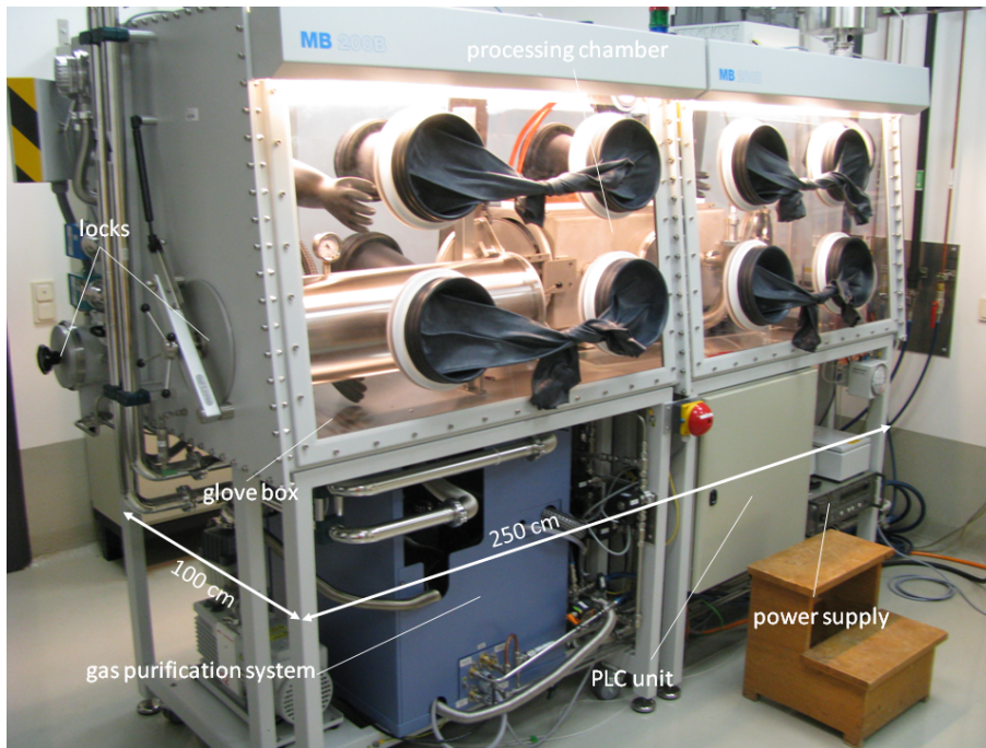
Figure 3.1: Full size reactor inside inert gas glove box in the LMU Physics Section. The whole full size reactor setup contains the sputtering reactor itself, a vacuum system, a gas system, a cooling system, a power supply, an control system, the autarkic gas purification/glove box system as well as several auxiliary systems.
