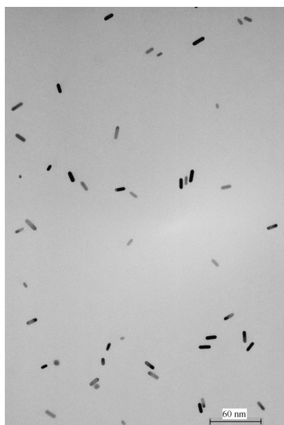
Figure 41: TEM image of rod-shaped Au particles produced by reducing \text{HAuCl}_4 with \text{NaBH}_4 . The particles were of 10 – 25 nm length (18 nm in average) and 3 – 7 nm width (5 nm in average).
