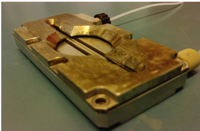
Figure 60: Image of the flow cell used for both qualitative and quantitative analysis of bacteria in aqueous environment.
