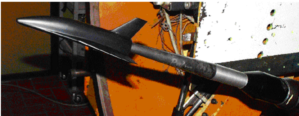
Figure 5.18: A photo of the EOS model for the TH2-D experiment.
