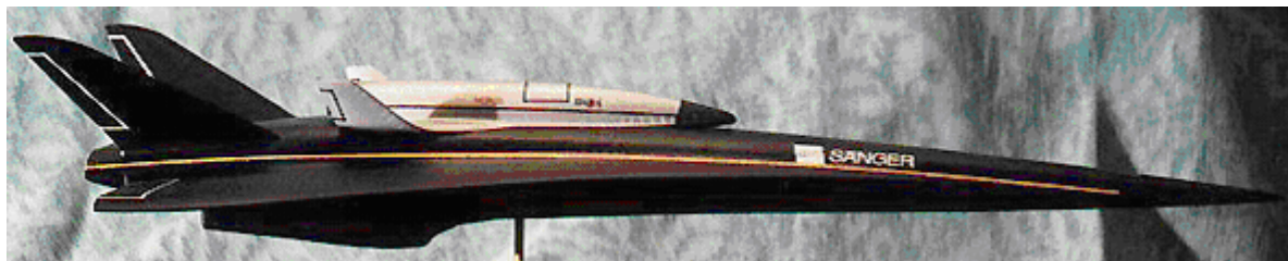
Figure 1.3: Configuration of the orbital and carrier stages in Sänger's concept.
