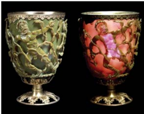
Figure 1.1 Images of the Lycurgus Cup (courtesy of the British Museum). The glass appears green in reflected light (left) and red in transmitted light (right), due to the presence of gold colloids.
